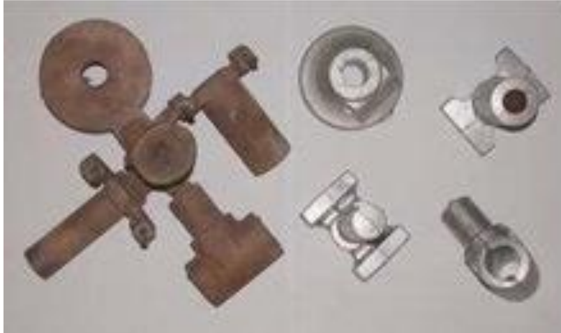
FIGURE - Two sets of castings (bronze and aluminum) from the above sand mold
