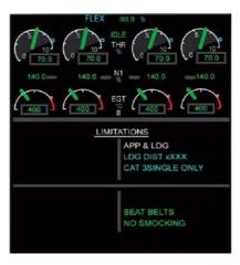
Fig 2.27. Engine/Warning display (by courtesy of Airbus).
