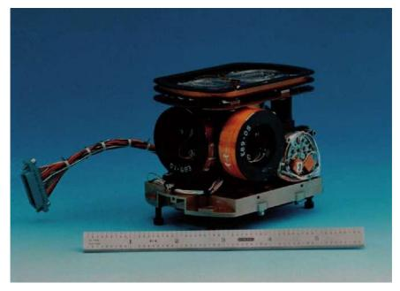
Fig 3.10. Fibre optic gyro inertial measuring unit (courtesy of Smiths Industries).
