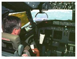
Fig2.3 Civil HUD installation – BAE Systems VGS HUD installed in a Boeing 737-800 series airliner (by courtesy of BAE Systems).
