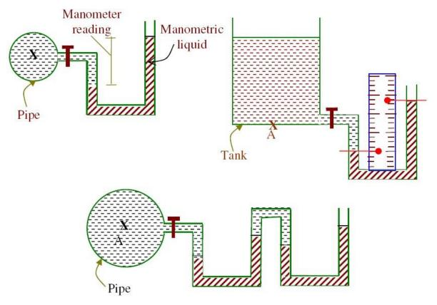
A U-tube manometers consists of a glass tube bent in U-Shape, one end of which is connected to gauge point and the other end is exposed to atmosphere. U-tube consists of a liquid of specific of gravity other than that of fluid whose pressure intensity is to be measured and is called manometric liquid.
