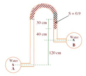
$$\begin{aligned} h_A - (190 \text{ x } 10^{-2}) + (0.3 \text{ x } 0.9) + (0.4) & 0.9 = h_B \\ h_A - h_B = 1.23 \text{ meters of water} \\ p_A - p_B = \gamma (h_A - h_B) = 9.81 \text{ x } 1.23 \\ p_A - p_B = 12.06 \text{ kPa} \\ p_A - p_B = 12.06 \text{ x } 10^3 \text{ N/m}^2 \end{aligned}$$
