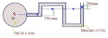
Let 'h<sub>M</sub>' be the pressure head at the point 'M' in m of water,
