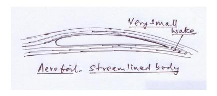
Fig. Flow over Bodies – Pressure Drag and Skin Friction Drag
