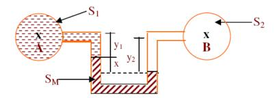
A differential U-tube manometer is used to measure pressure difference between any two points. It consists of a U-tube containing heavier manometric liquid, the two limbs of which are connected to the gauge points between which the pressure difference is required. U-tube differential manometers can also be used for gases. By writing the gauge equation for the system pressure difference can be determined.
