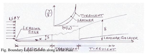
Up to a certain length along the plate from the leading edge, boundary layer thickness increases and the boundary layer exhibits the characteristics of a laminar flow irrespective of whether the incoming flow is laminar or turbulent. – This is known as laminar boundary layer.
