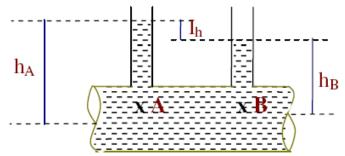
The arrangement consists of two pizometers at the two points between which the pressure difference is required. The liquid will rise in both the piezometers. The difference in elevation of liquid levels can be recorded and the pressure difference can be calculated.
