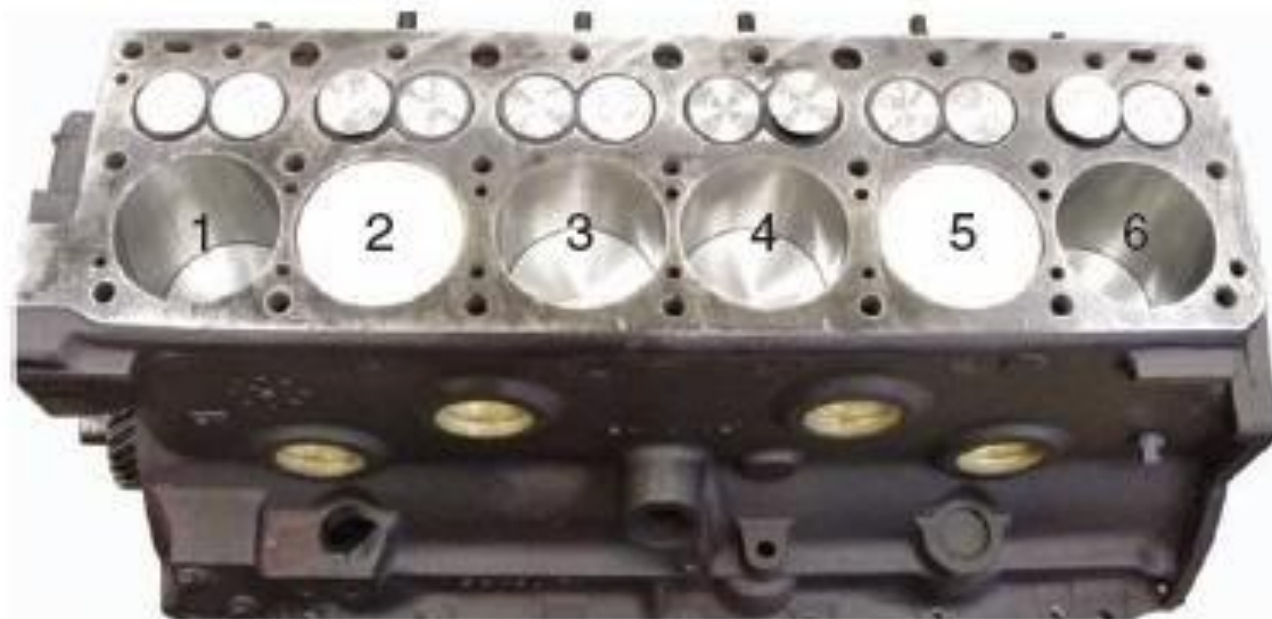
Figure 16.5 This vintage L-head in-line six-cylinder engine shows companion cylinder pairings. The pistons in cylinders 1 and 6, 2 and 5, and 3 and 4 go up and down together.
