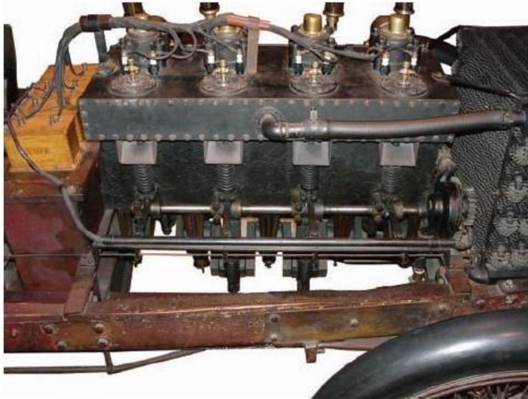
Figure 1.24 This early engine had no valve cover or oil pan. Lubricant was provided by drip oil.
