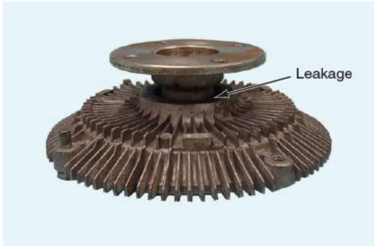
Figure 21.38 Some trucks and SUVs use a belt-driven fan clutch. Inspect it for leakage.
