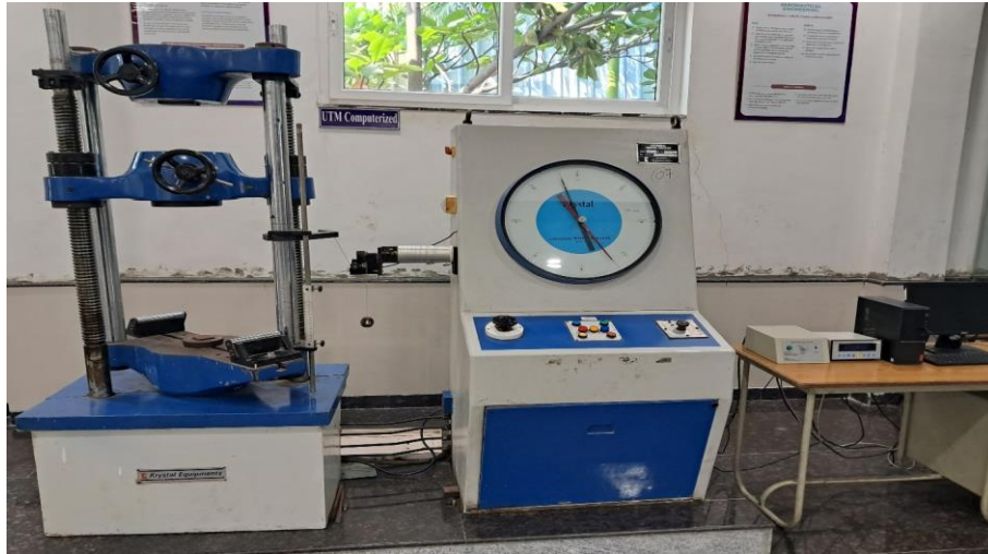
Fig. 8.1: UTM Machine for finding young's modulus
