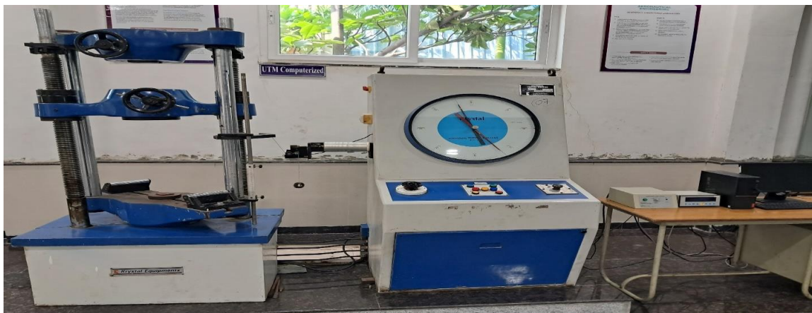
Fig. 7.2: UTM machine for finding shear stress
