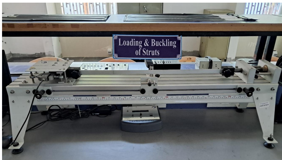
Fig. 3.1: Loading and buckling of struts equipment for compression test
