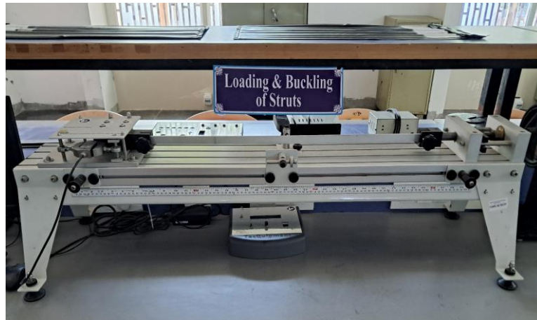
Fig. 2.1: Loading and buckling of struts equipment
