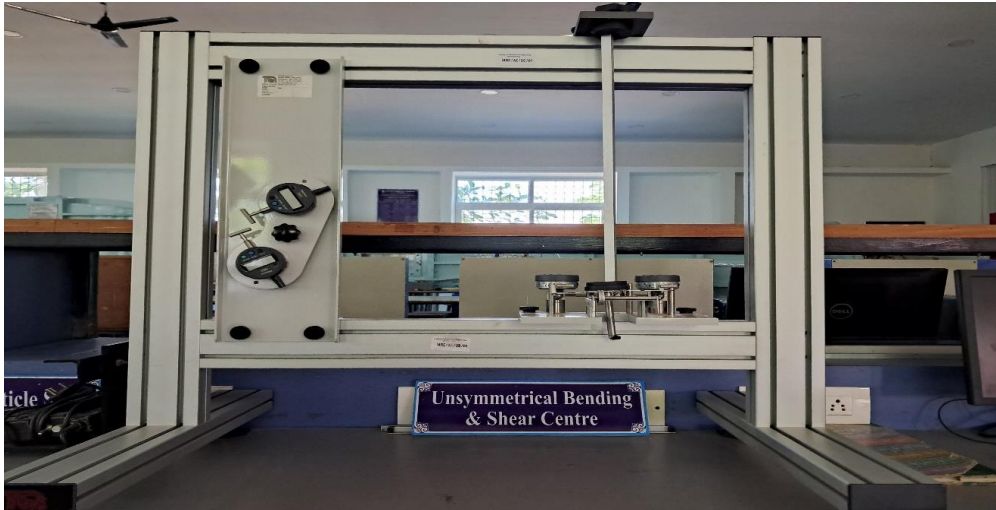
Fig. 5.1: Equipment for determination of shear centre of an open section beam
