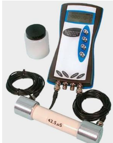
Fig.10.2 Ultrasonic Pulse Velocity Tester
