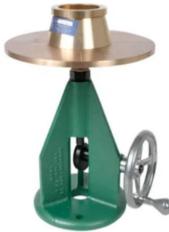
Fig.12.2 Flow table test apparatus
