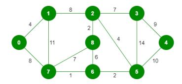
The graph contains 9 vertices and 14 edges. So, the minimum spanning tree formed will be having (9 - 1) = 8 edges.
