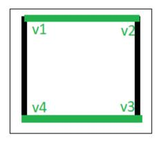
Edge colorings are one of several different types of graph coloring problems. The above figure of a Graph shows an edge coloring of a graph by the colors green and black, in which no adjacent edge have the same color.
