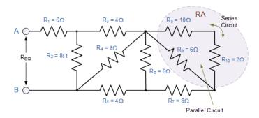
$$R_A = \frac{R_9 \times (R_8 + R_{10})}{R_9 + R_8 + R_{10}} = \frac{6 \times (10 + 2)}{6 + 10 + 2} = 4\Omega$$
