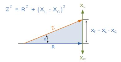
The impedance Z of a series RLC circuit depends upon the angular frequency,  $\omega$  as do  $X_L$  and  $X_C$  If the capacitive reactance is greater than the inductive reactance,  $X_C > X_L$  then the overall circuit reactance is capacitive giving a leading phase angle.
