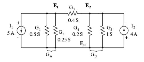
The parallel conductances (resistors) may be combined by addition of the conductances. Though, we will not redraw the circuit. The circuit is ready for application of the node voltage method.
