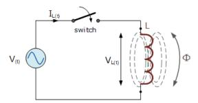
This simple circuit above consists of a pure inductance of L Henries ( H ), connected across a sinusoidal voltage given by the expression:  $V(t) = V_{max} \sin \omega t$ . When the switch is closed this sinusoidal voltage will cause a current to flow and rise from zero to its maximum value. This rise or change in the current will induce a magnetic field within the coil which in turn will oppose or restrict this change in the current.
