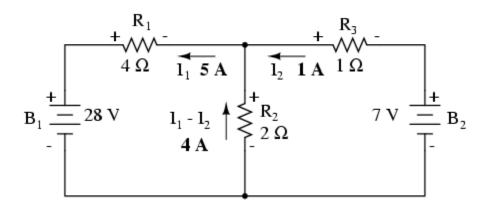
A current of 4 amps through  $R_2$ 's resistance of 2  $\Omega$  gives us a voltage drop of 8 volts (E=IR), positive on the top and negative on the bottom.
