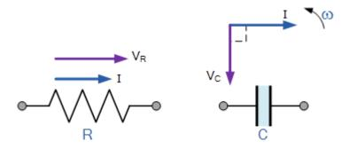
Both the voltage and current vectors for an AC Resistance are in phase with each other and therefore the voltage vector  $V_R$  is drawn superimposed to scale onto the current vector. Also we know that the current leads the voltage (ICE) in a pure AC capacitance circuit, therefore the voltage vector  $V_C$  is drawn  $90^\circ$  behind (lagging) the current vector and to the same scale as  $V_R$  as shown.
