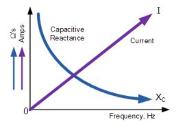
Capacitive reactance of a capacitor decreases as the frequency across its plates increases. Therefore, capacitive reactance is inversely proportional to frequency. Capacitive reactance opposes current flow but the electrostatic charge on the plates (its AC capacitance value) remains constant.
