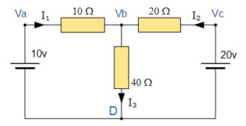
In the above circuit, node D is chosen as the reference node and the other three nodes are assumed to have voltages, Va, Vb and Vc with respect to node D. For example;
