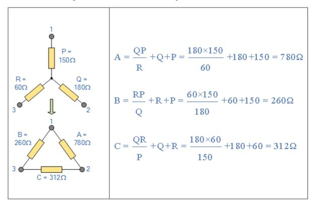
Both Star Delta Transformation and Delta Star Transformation allows us to convert one type of circuit connection into another type in order for us to easily analyse the circuit. These transformation techniques can be used to good effect for either star or delta circuits containing resistances or impedances.
