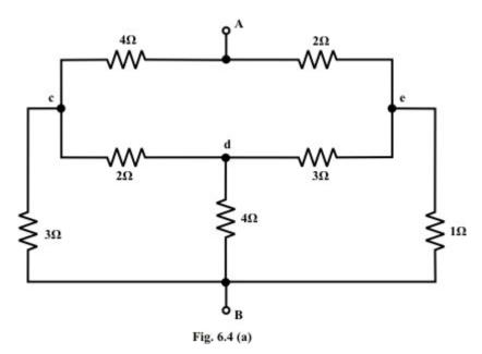
A ' $\Delta$ ' is substituted for the 'Y' between points c, d, and e as—shown in fig.6.4(b); then unknown resistances value for Y to  $\Delta$  transformation—are computed below.
