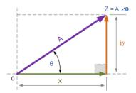
As the polar representation of a point is based around the triangular form, we can use simple geometry of the triangle and especially trigonometry and Pythagoras's Theorem on triangles to find both the magnitude and the angle of the complex number. As we remember from school, trigonometry deals with the relationship between the sides and the angles of triangles so we can describe the relationships between the sides as:
