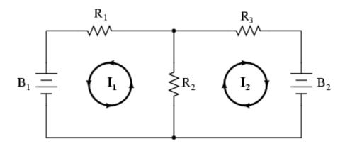
The choice of each current's direction is entirely arbitrary, just as in the Branch Current method, but the resulting equations are easier to solve if the currents are going the same direction through intersecting components (note how currents  $I_1$  and  $I_2$  are both going "up" through resistor  $R_2$ , where they "mesh," or intersect). If the assumed direction of a mesh current is wrong, the answer for that current will have a negative value.
