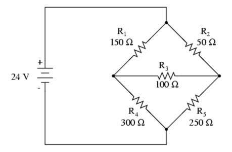
Since the ratios of  $R_1/R_4$  and  $R_2/R_5$  are unequal, we know that there will be voltage across resistor  $R_3$ , and some amount of current through it. As discussed at the beginning of this chapter, this type of circuit is irreducible by normal series-parallel analysis, and may only be analyzed by some other method.
