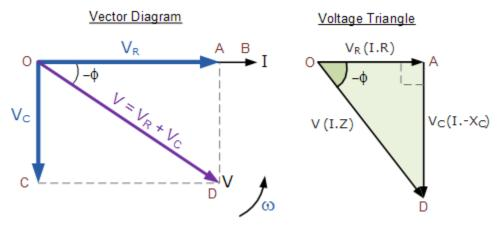
In the vector diagram above, line OB represents the horizontal current reference and line OA is the voltage across the resistive component which is in-phase with the current. Line OC shows the capacitive voltage which is 90° behind the current therefore it can still be seen that the current leads the purely capacitive voltage by 90°. Line OD gives us the resulting supply voltage.
