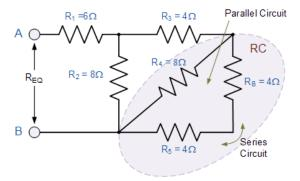
This resistive value of  $8\Omega$  is now in parallel with  $R_4$  and can be calculated as  $R_C$  as shown.
