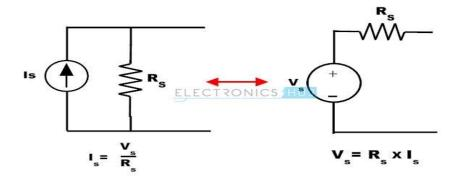
In the above figure, a current source is converted into a voltage source by placing resistance Rs in series with a voltage source and the value of the voltage source is calculated as,
