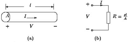
Figure 1.2: Ohm's law. (a) Metal wire; (b) circuit symbol
