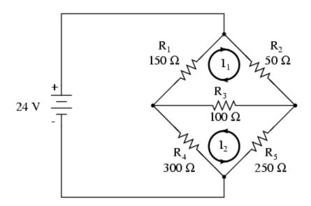
The directions of these mesh currents, of course, is arbitrary. However, two mesh currents is not enough in this circuit, because neither  $I_1$  nor  $I_2$  goes through the battery. So, we must add a third mesh current,  $I_3$ :
