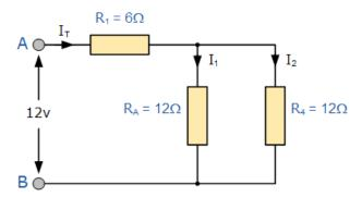
So our circuit now has a single resistor  $R_A$  in "PARALLEL" with the resistor  $R_4$ . Using our resistors in parallel equation we can reduce this parallel combination to a single equivalent resistor value of  $R_{\text{(combination)}}$  using the formula for two parallel connected resistors as follows.
