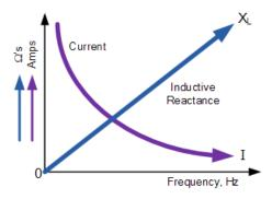
The inductive reactance of an inductor increases as the frequency across it increases therefore inductive reactance is proportional to frequency ( $X_L \alpha f$ ) as the back emf generated in the inductor is equal to its inductance multiplied by the rate of change of current in the inductor.
