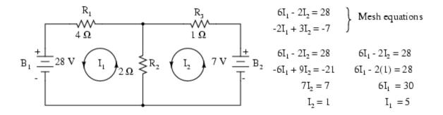
The currents  $I_1 = 5$  A, and  $I_2 = 1$  A are both positive. They both flow in the direction of the counterclockwise loops. This compares with previous results.
