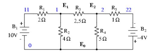
A voltage source in series with a resistance must be replaced by an equivalent current source in parallel with the resistance. We will write KCL equations for each node. The right hand side of the equation is the value of the current source feeding the node.
