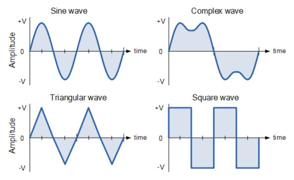
Figure AC waveforms
