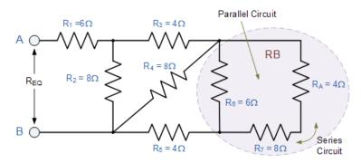
This resistive value of  $12\Omega$  is now in parallel with  $R_6$  and can be calculated as  $R_B$ .
