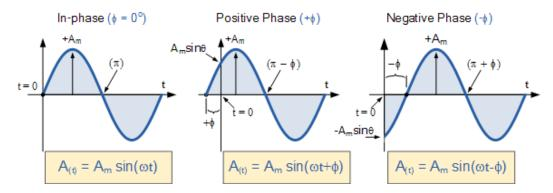
Firstly, lets consider that two alternating quantities such as a voltage, v and a current, ihave the same frequency f in Hertz. As the frequency of the two quantities is the same the angular velocity,  $\omega$  must also be the same. So at any instant in time we can say that the phase of voltage, v will be the same as the phase of the current, i.
