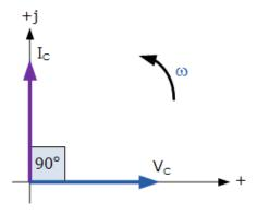
So for a pure capacitor,  $V_C$  "lags"  $I_C$  by  $90^\circ$ , or we can say that  $I_C$  "leads"  $V_C$  by  $90^\circ$ .
