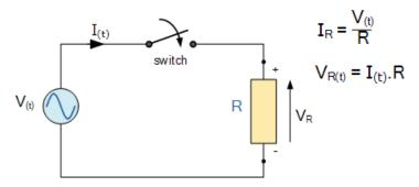
When the switch is closed, an AC voltage, V will be applied to resistor, R. This voltage will cause a current to flow which in turn will rise and fall as the applied voltage rises and falls sinusoidally. As the load is a resistance, the current and voltage will both reach their maximum or peak values and fall through zero at exactly the same time, i.e. they rise and fall simultaneously and are therefore said to be "*in-phase*".
