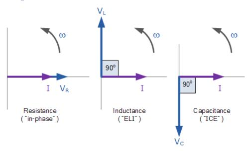
This means then that we can not simply add together  $V_R$ ,  $V_L$  and  $V_C$  to find the supply voltage,  $V_S$  across all three components as all three voltage vectors point in different directions with regards to the current vector. Therefore we will have to find the supply voltage,  $V_S$  as the **Phasor Sum** of the three component voltages combined together vectorially.
