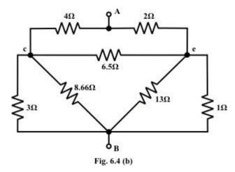
Next we transform ' $\Delta$ ' connected 3-terminal resistor to an equivalent 'Y' connected network between points ' $\Delta$ '; ' $\Delta$ ' and ' $\Delta$ ' (see fig.6.4(b)) and the corresponding Y connected resistances value are obtained using the following expression. Simplified circuit after conversion is shown in fig
