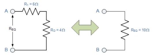
Then the complex combinational resistive network above comprising of ten individual resistors connected together in series and parallel combinations can be replaced with just one single equivalent resistance ( REQ ) of value  $10\Omega$ .
