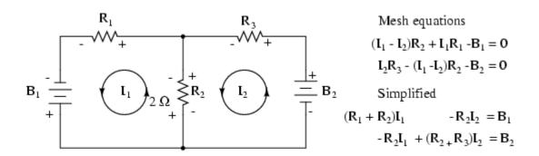
Once rearranged, we may write equations by inspection. The signs of the coefficients follow a fixed pattern in the pair above, or the set of three in the rules below.
