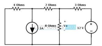
• In the circuit there are two areas where we can apply the source transformation since current source has a parallel resistor and voltage source has a series resistor as shown in figure. So these configurations are necessary requirements to apply the source transformation.
