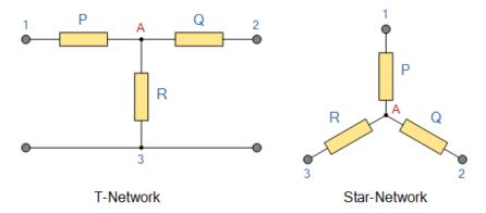
As we have already seen, we can redraw the T resistor network above to produce an electrically equivalent **Star** or Y type network. But we can also convert a Pi or  $\pi$  type resistor network into an electrically equivalent **Delta** or  $\Delta$  type network as shown below.
