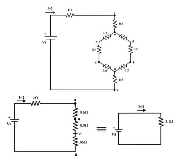
The source  $V_s$  that delivers 2A current through the circuit can be obtained as  $V_s = I \times 3.2 = 2 \times 3.1 = 6.2 Volts$ .
