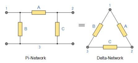
Having now defined exactly what is a **Star** and **Delta** connected network it is possible to transform the Y into an equivalent  $\Delta$  circuit and also to convert a  $\Delta$  into an equivalent Y circuit using a the transformation process.
