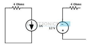
• Place the above voltage source with a series resistance in the circuit, then we get below figure.
