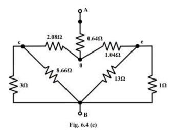
$$R_{_{Ao}} = \frac{4 \times 2}{4 + 2 + 6.5} = 0.64 \Omega \, ; \ \ R_{_{co}} = \frac{4 \times 6.5}{4 + 2 + 6.5} = 2.08 \Omega \, ; \ \ R_{_{eo}} = \frac{6.5 \times 2}{4 + 2 + 6.5} = 1.04 \Omega \, ;$$
