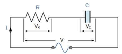
In the RC series circuit above, we can see that the current flowing into the circuit is common to both the resistance and capacitance, while the voltage is made up of the two component voltages,  $V_R$  and  $V_C$ . The resulting voltage of these two components can be found mathematically but since vectors  $V_R$  and  $V_C$  are 90° out-of-phase, they can be added vectorially by constructing a vector diagram.
