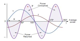
In the positive half of the voltage waveform between the angle of 0o and 90o, the inductor current is negative while the supply voltage is positive. Therefore, the volts and ampere product gives a negative power as negative times a positive equals a negative. Between 90o and 180o, both current and voltage waveforms are positive in value resulting in positive power. This positive power indicates that the coil is consuming electrical energy from the supply.
