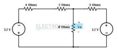
• Resistors 4 ohms and 2 ohms are in series, hence the total series resistance will be 6 ohms as shown below.
