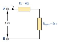
We can see that the two remaining resistances,  $R_1$  and  $R_{\text{(comb)}}$  are connected together in a "SERIES" combination and again they can be added together (resistors in series) so that the total circuit resistance between points A and B is therefore given as:
