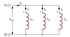
In the previous series inductors tutorial, we saw that the total inductance,  $L_T$  of the circuit was equal to the sum of all the individual inductors added together. For inductors in parallel the equivalent circuit inductance  $L_T$  is calculated differently.
