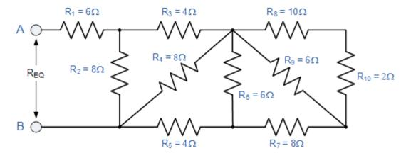
Again, at first glance this resistor ladder network may seem a complicated task, but as before it is just a combination of series and parallel resistors connected together. Starting from the right hand side and using the simplified equation for two parallel resistors, we can find the equivalent resistance of the R8 to R10 combination and call it RA.
