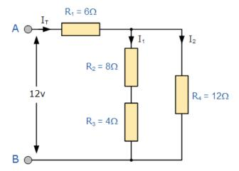
At first glance this may seem a difficult task, but if we look a little closer we can see that the two resistors,  $R_2$  and  $R_3$  are actually both connected together in a "SERIES" combination so we can add them together to produce an equivalent resistance the same as we did in the series resistor tutorial. The resultant resistance for this combination would therefore be:
