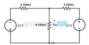
• Again the voltage source of 12V with series resistor 6 ohms can be transformed into a current source. Therefore consider to transform it.
