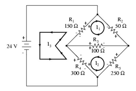
Notice something very important here: at resistor  $R_4$ , the polarities for the respective mesh currents do not agree. This is because those mesh currents ( $I_2$  and  $I_3$ ) are going through  $R_4$  in different directions. This does not preclude the use of the Mesh Current method of analysis, but it does complicate it a bit. Though later, we will show how to avoid the  $R_4$  current clash. (See Example below)
