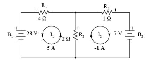
The solution of -1 amp for  $I_2$  means that our initially assumed direction of current was incorrect. In actuality,  $I_2$  is flowing in a counter-clockwise direction at a value of (positive) 1 amp:
