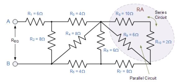
$$R_{A} = \frac{R_{9} \times (R_{8} + R_{10})}{R_{9} + R_{8} + R_{10}} = \frac{6 \times (10 + 2)}{6 + 10 + 2} = 4\Omega$$
