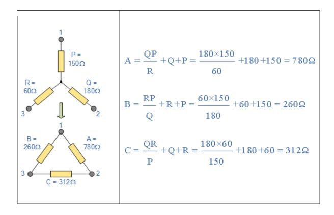
Both Star Delta Transformation and Delta Star Transformation allows us to convert one type of circuit connection into another type in order for us to easily analyse the circuit. These transformation techniques can be used to good effect for either star or delta circuits containing resistances or impedances.
