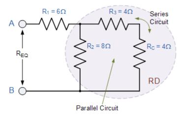
This resistive value of  $8\Omega$  is now in parallel with R2 from which we can calculated RD as:
