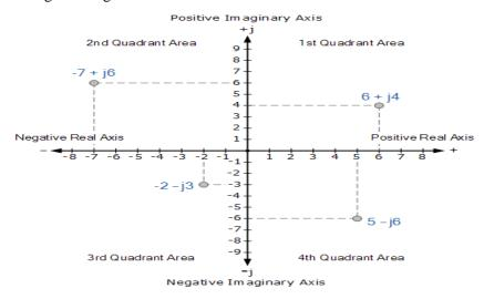
On the Argand diagram, the horizontal axis represents all positive real numbers to the right of the vertical imaginary axis and all negative real numbers to the left of the vertical imaginary axis. All positive imaginary numbers are represented above the horizontal axis while all the negative imaginary numbers are below the horizontal real axis. This then produces a two dimensional complex plane with four distinct quadrants labelled, QI, QII, QIII, and QIV.
