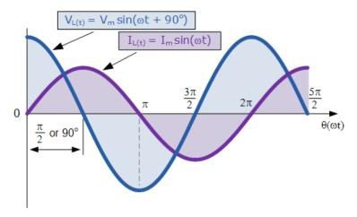
This effect can also be represented by a phasor diagram were in a purely inductive circuit the voltage "LEADS" the current by 90°. But by using the voltage as our reference, we can also say that the current "LAGS" the voltage by one quarter of a cycle or 90° as shown in the vector diagram below.
