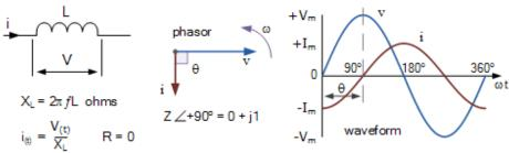
The waveforms above show us the instantaneous voltage and instantaneous current across a purely inductive coil as a function of time. Maximum current,  $I_m$  occurs at one full quarter of a cycle (90°) after the maximum (peak) value of the voltage. Here the current is shown with its negative maximum value at the start of the voltage cycle and passes through zero increasing to its positive maximum value when the voltage waveform is at its maximum value at  $90^\circ$ .
