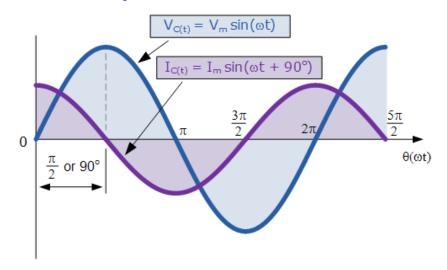
During the second half cycle 180° to 360°, the supply voltage reverses direction and heads towards its negative peak value at 270°. At this point the potential difference across the plates is neither
