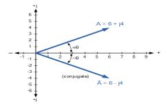
The sum of a complex number and its complex conjugate will always be a real number as we have seen above. Then the addition of a complex number and its conjugate gives the result as a real number or active component only, while their subtraction gives an imaginary number or reactive
