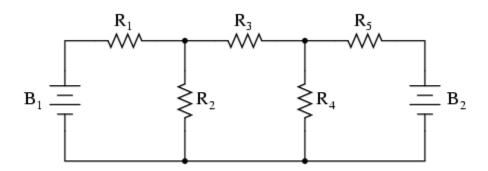
To solve this network using Branch Currents, we'd have to establish five variables to account for each and every unique current in the circuit ( $I_1$  through  $I_5$ ). This would require five equations for solution, in the form of two KCL equations and three KVL equations (two equations for KCL at the nodes, and three equations for KVL in each loop):
