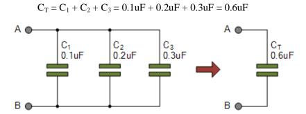
One important point to remember about parallel connected capacitor circuits, the total capacitance ( $C_T$ ) of any two or more capacitors connected together in parallel will always be **GREATER** than the value of the largest capacitor in the group as we are adding together values. So in our example above  $C_T = 0.6 uF$  whereas the largest value capacitor is only 0.3 uF.
