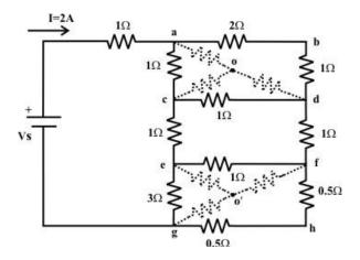
Convert the three terminals  $\Delta$ -network (a-c-d & e-f-g) into an equivalent Y-connected network. Consider the  $\Delta$ -connected network 'a-c-d' and the corresponding equivalent Y-connected resistor values are given as
