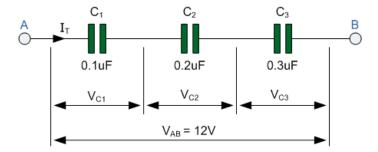
In the previous parallel circuit we saw that the total capacitance,  $C_T$  of the circuit was equal to the sum of all the individual capacitors added together. In a series connected circuit however, the total or equivalent capacitance  $C_T$  is calculated differently.
