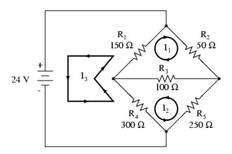
Here, I have chosen  $I_3$  to loop from the bottom side of the battery, through  $R_4$ , through  $R_1$ , and back to the top side of the battery. This is not the only path I could have chosen for  $I_3$ , but it seems the simplest.
