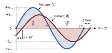
The voltage waveform above starts at zero along the horizontal reference axis, but at that same instant of time the current waveform is still negative in value and does not cross this reference axis until 30° later. Then there exists a **Phase difference** between the two waveforms as the current cross the horizontal reference axis reaching its maximum peak and zero values after the voltage waveform.
