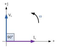
So for a pure loss less inductor, V<sub>L</sub> "leads" I<sub>L</sub> by 90°, or we can say that I<sub>L</sub> "lags" V<sub>L</sub> by 90°.
