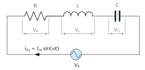
The series RLC circuit above has a single loop with the instantaneous current flowing through the loop being the same for each circuit element. Since the inductive and capacitive reactance's  $X_L$  and  $X_C$  are a function of the supply frequency, the sinusoidal response of a series RLC circuit will therefore vary with frequency, f. Then the individual voltage drops across each circuit element of R, L and C element will be "out-of-phase" with each other as defined by:
