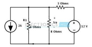
• On the right hand side, there is a voltage source with a 3 ohms resistor so this can be transformed into a current source by placing a 3 ohm resistor in parallel with a current source and this current source value is calculated as
