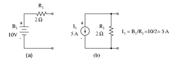
Replacing voltage sources and associated series resistors with equivalent current sources and parallel resistors yields the modified circuit. Substitute resistor conductances in siemens for resistance in ohms.
