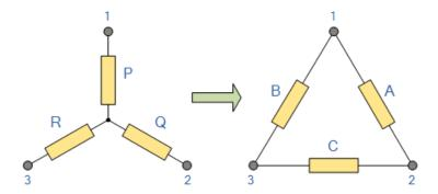
The value of the resistor on any one side of the delta,  $\Delta$  network is the sum of all the two-product combinations of resistors in the star network divide by the star resistor located "directly opposite" the delta resistor being found. For example, resistor A is given as:
