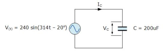
The voltage across the capacitor will be the same as the supply voltage. Converting this time domain value into polar form gives us:  $V_C = 240 \ \angle -20^\circ$  (v). The capacitive reactance will be:  $X_C = 1/(\ \omega.200 uF)$ . Then the current flowing into the capacitor can be found using Ohms law as:
