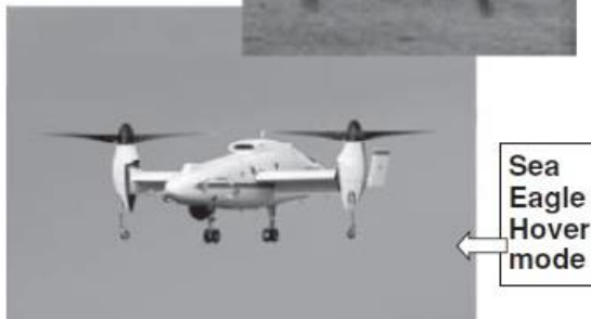
Figure 3.12 Medium-range VTOL UAV systems: Seagull (Reproduced by permission of Beijing UAA) and Sea Eagle (Reproduced by permission of Bell Helicopter Textron Inc.)
