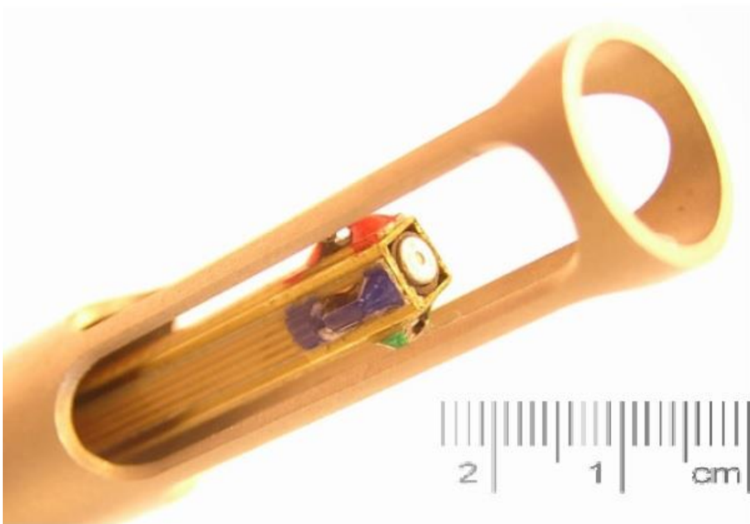
Figure 5.10: An acoustic vector sensor consisting of a sound pressure microphone and three orthogonally placed Microflow sensors
