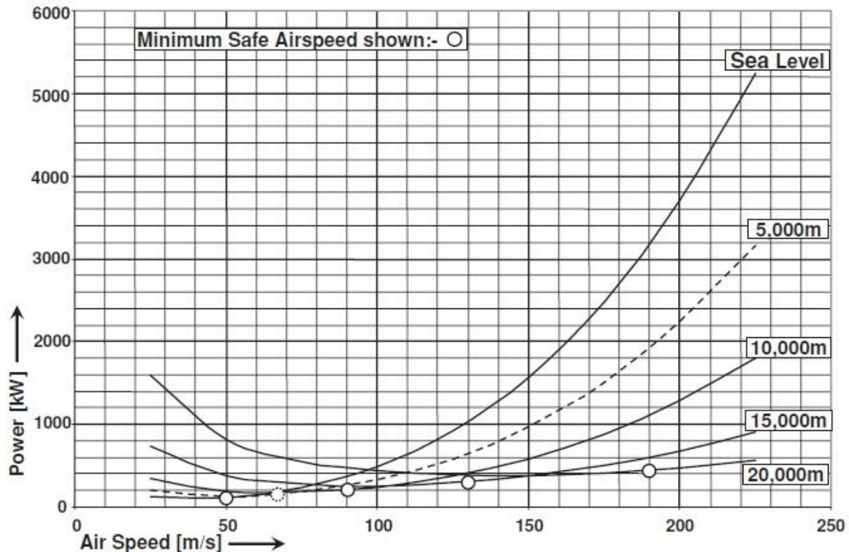
Figure 3.7: HALE UAV: power required to maintain height. Variation with airspeed and altitude – 81.8 kN AUW, ISA conditions
