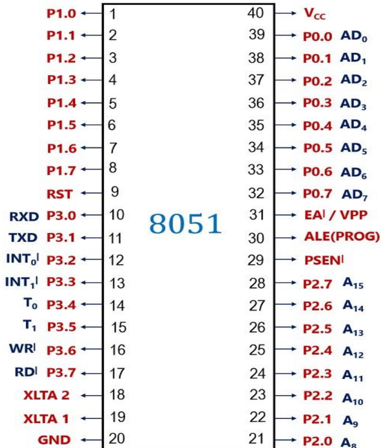
Pin diagram of 8051 Microcontroller
