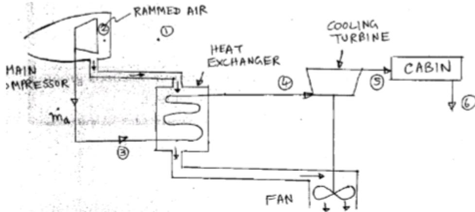
Fig. Simple Air Cooling System
