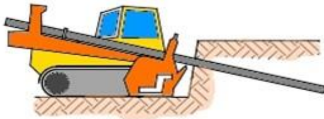
STEP 2. DRILL NAIL HOLE
