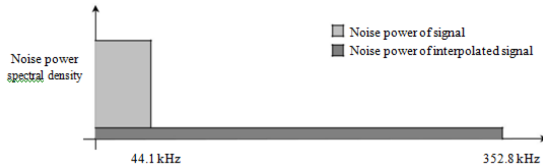
Figure :Illustration of noise power spectral density reduction due to oversampling.
