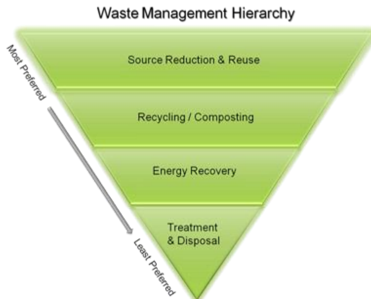
Fig.3.7. Non-Hazardous Materials and Waste Management Hierarchy
