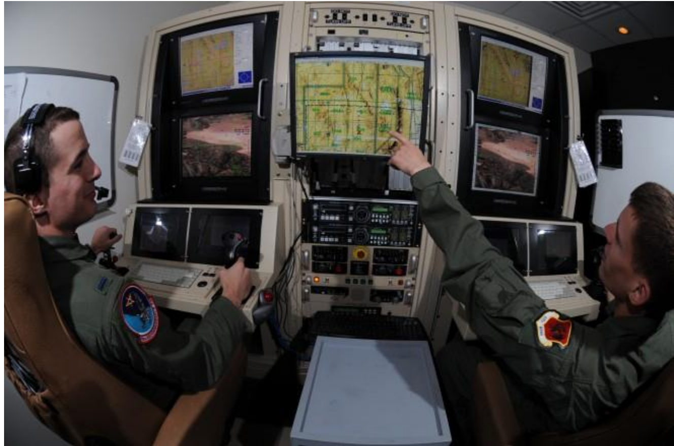
Figure 1.3 .GCS - Ground control station
