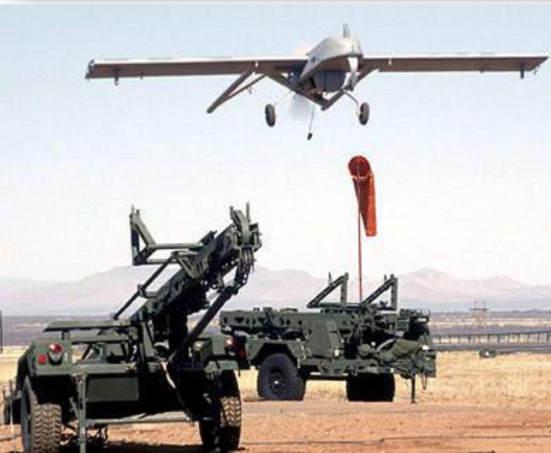
Hydraulic rail launcher
