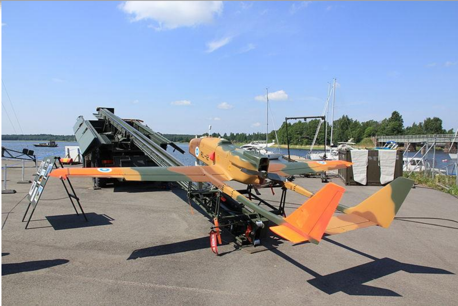
Figure 3.17 : Ranger UAV by RUAG, Switzerland , uses hydraulic launcher
