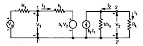
Transistor amplifier in its h-parameter model
