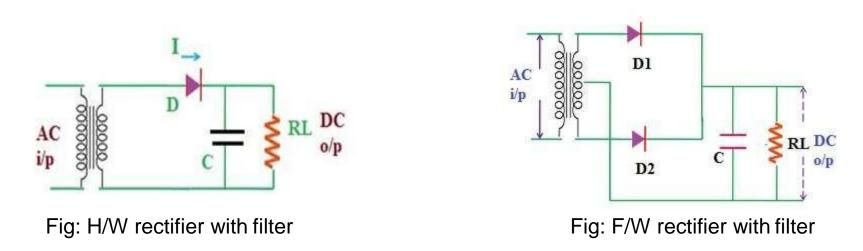
•In full wave rectifier circuit using a capacitor filter, the capacitor C is located across the RL load resistor. The working of this rectifier is almost the same as a half wave rectifier.
