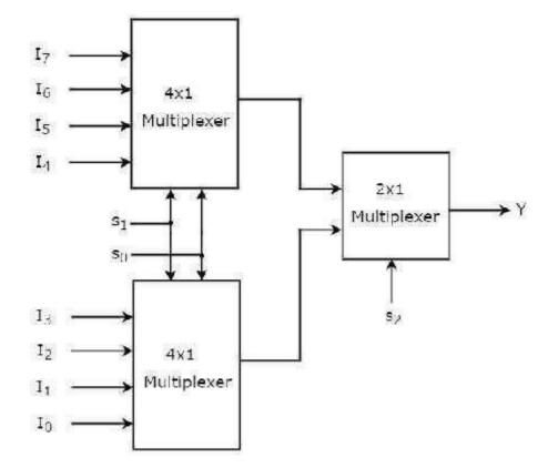
Fig 3: 8x1 Multiplexer diagram
