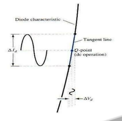
Fig: Dynamic resistance curve
