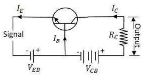
Fig.4: NPN Transistor in CB Configuration
