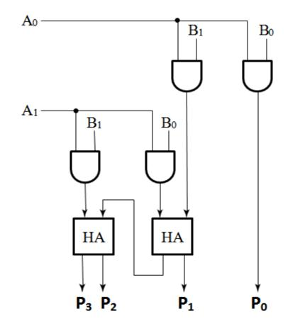
Fig 1: 2 x 2 multiplier array
