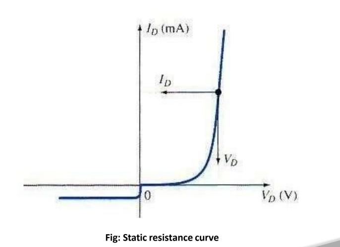
Static resistance is using dc input.
