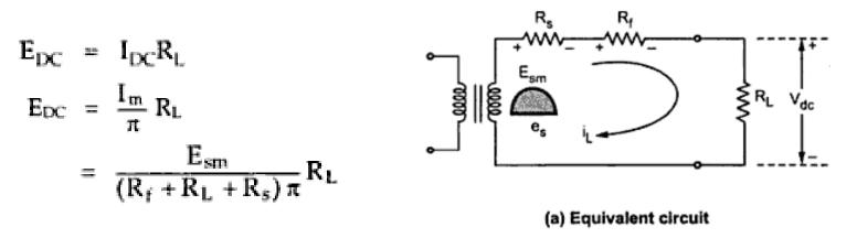
But as  $R_f$  and  $R_s$  are small compared to  $R_L$ ,  $(R_f + R_s)/R_L$  is negligibly small compared to 1. So neglecting it we get,
