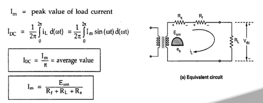
where  $R_s =$  resistance of secondary winding of transformer. If  $R_s$  is not given it should be neglected while calculating  $I_m$ .
