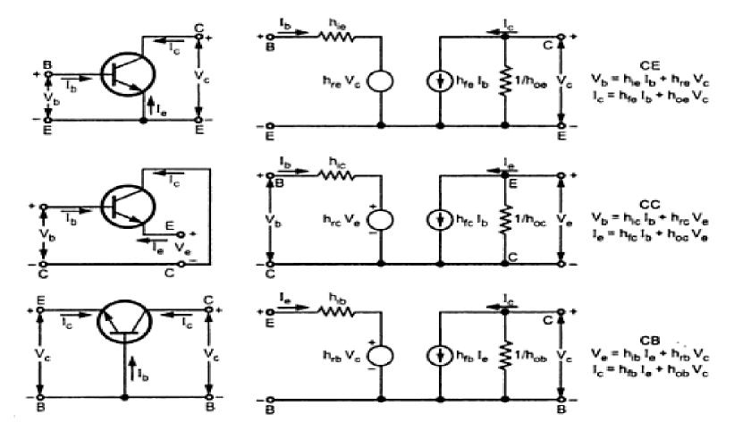
Transistor configurations and their hybrid models
