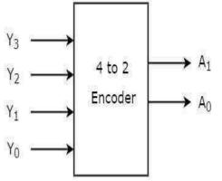
Fig 1:block diagram of 4x2encoder
