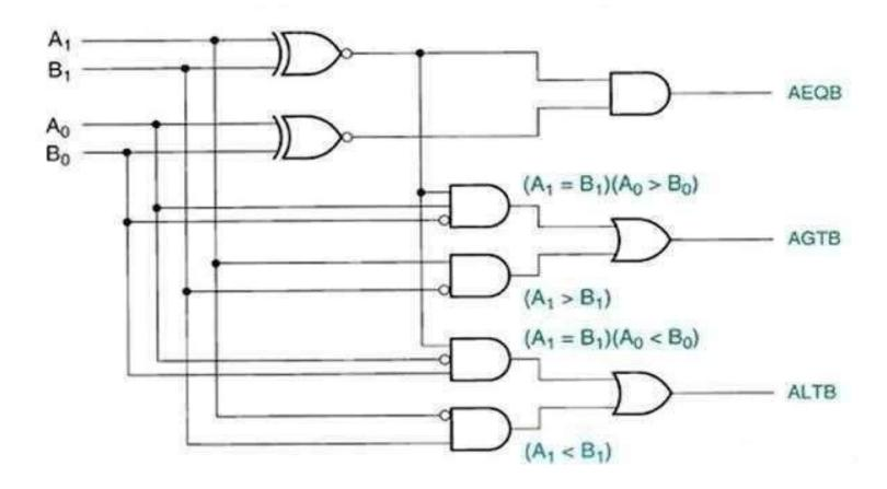
Fig 5:Logic diagram of 2-bitcomparator
