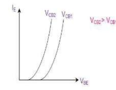
Fig.5: CB Configuration I/P Characteristics
