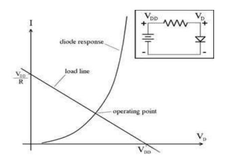
A load line is a line drawn on the characteristic curve, a graph of the current vs. voltage in a nonlinear device like a diode.
