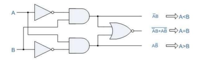
Fig 2:Logic diagram of 1-bit comparator
