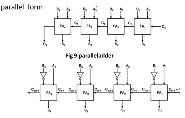
Fig 10:parallel subtractor
