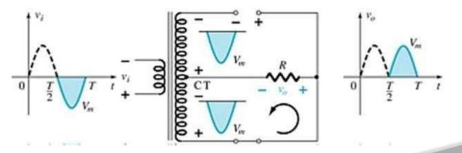
Current Flow during the negative half of the input cycle
