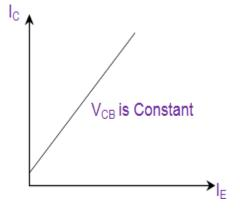
Fig.7: CB Configuration Current Transfer Characteristics
