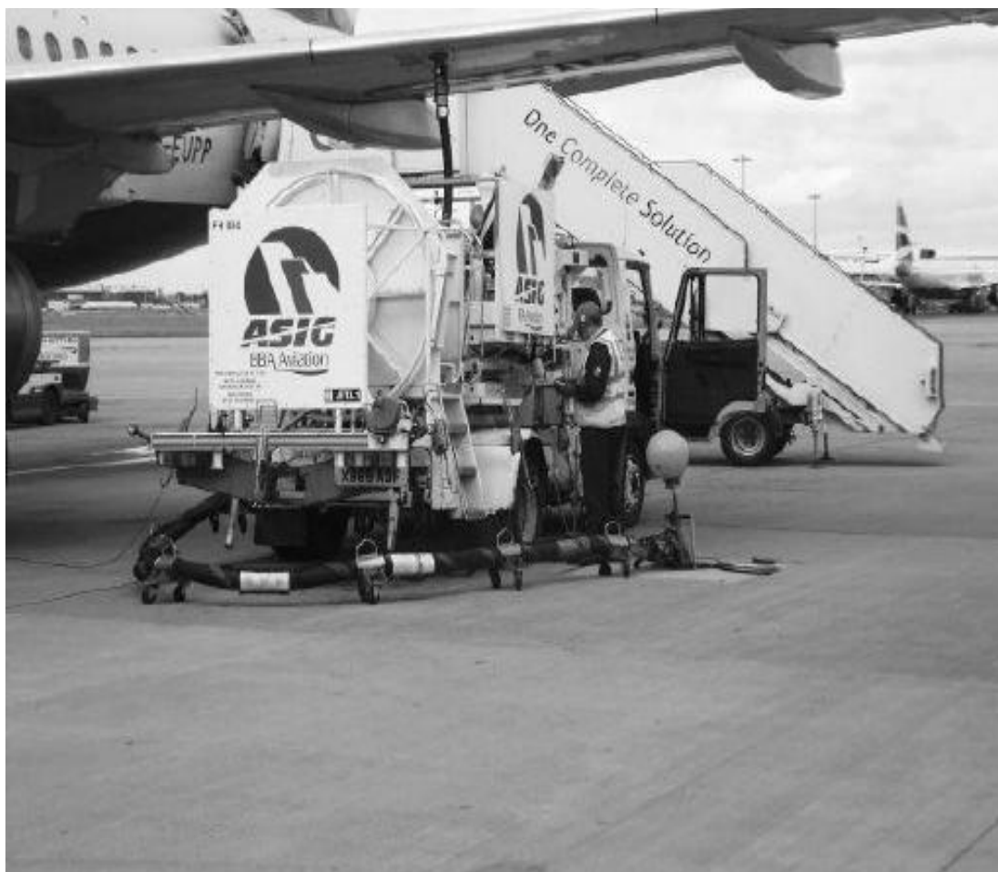
Fig.3.8 Mobile aircraft fuel dispenser for fueling from apron hydrant system.
