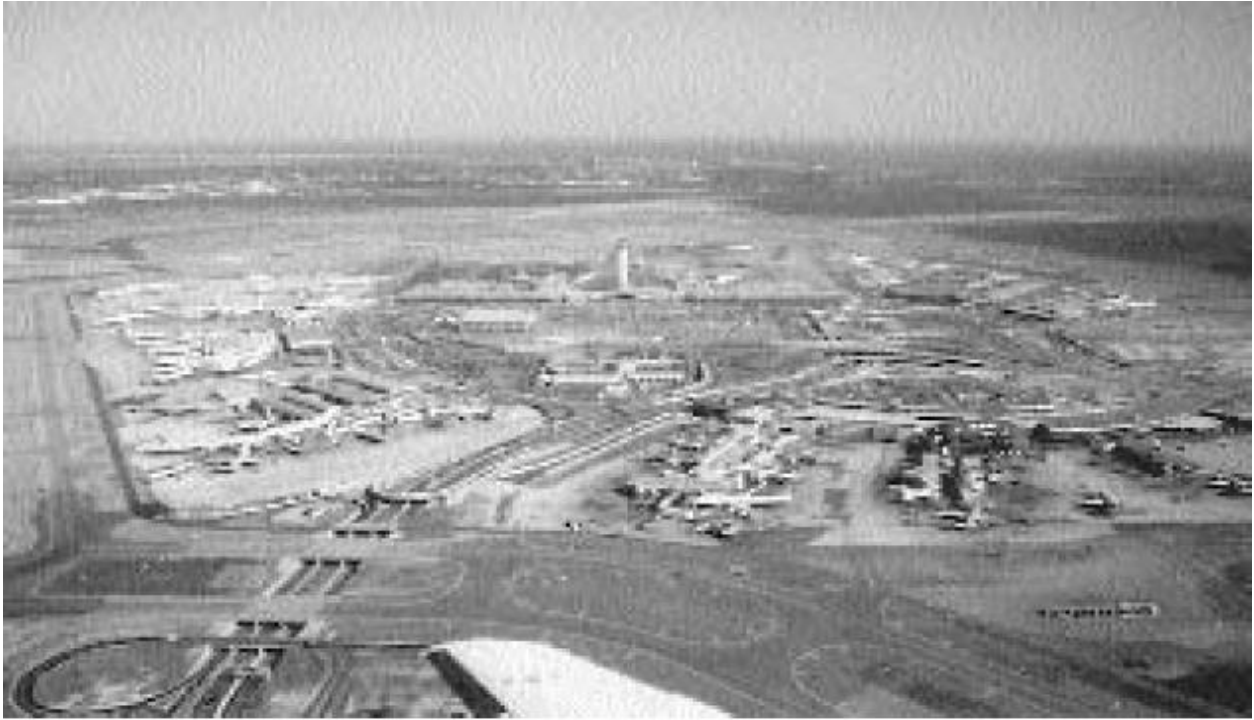
Fig 3.12 Combined unit terminal
