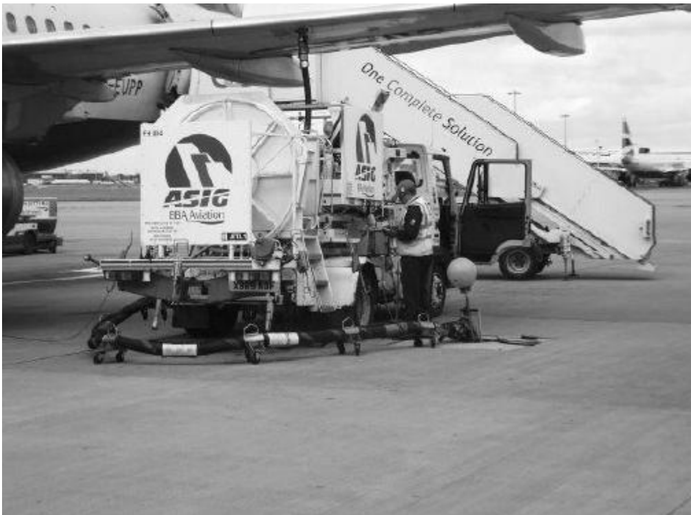
Fig 2.10 Mobile aircraft fuel dispenser for fueling from apron hydrant system.
