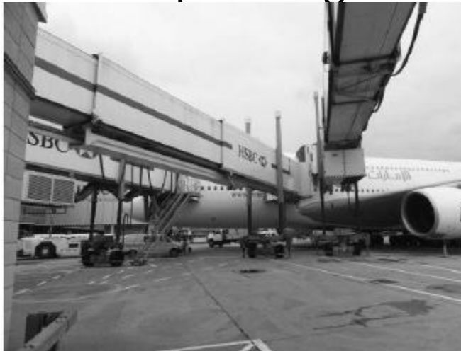
Three-loading-bridge configuration serving an A380
