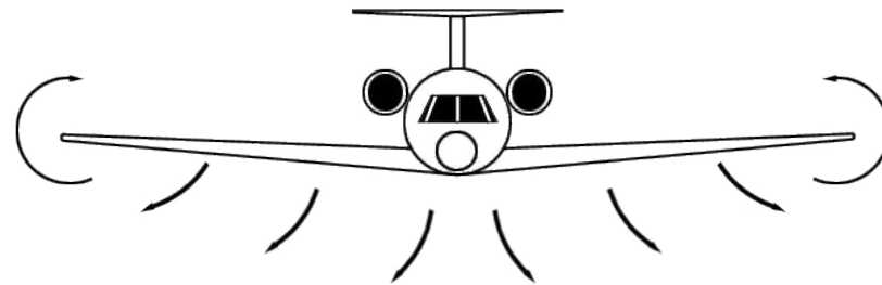
Vortices fully formed at altitude
