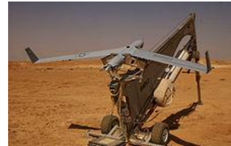
ScanEagle reconnaissance UAV on its catapult launcher
