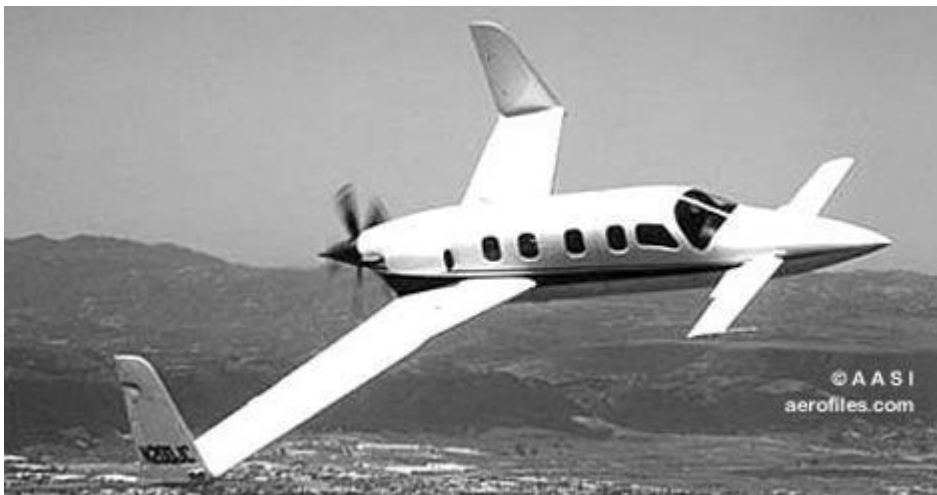
Fig 1.14: Pusher configuration of Jetcruzer 500, AASI airplane.
