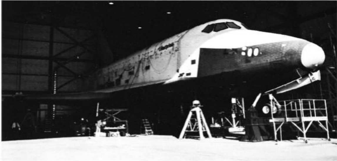
Fig. Vibration testing of the space shuttle Enterprise.
