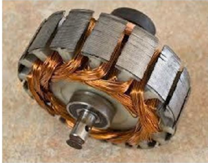
Figure 2.2 Armature core (rotor)
