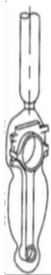
1. Blank (bar) 2. Edging 3. Blocking 4. Finishing 5. Trimming
