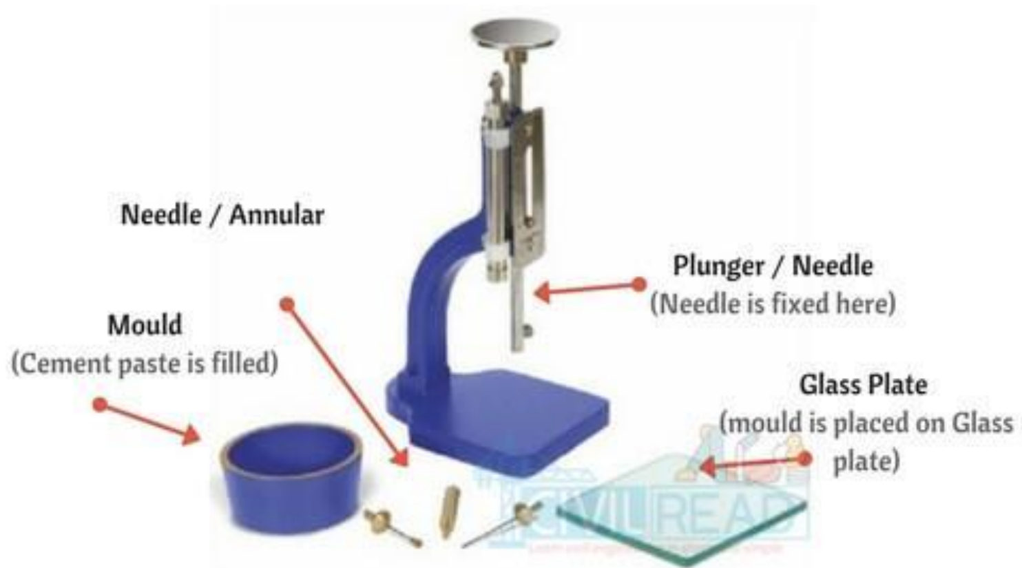
VICAT Apparatus with details
