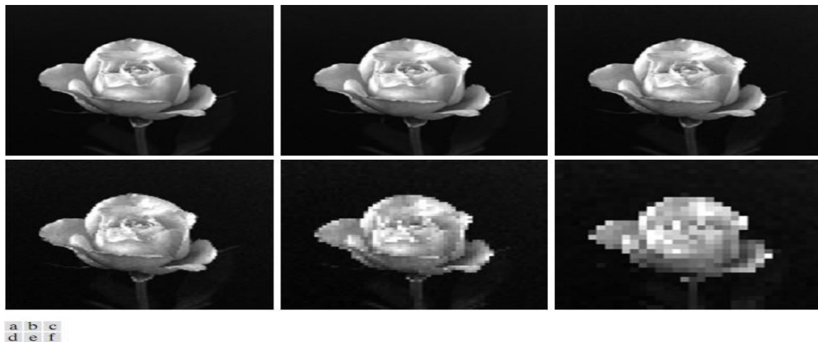
Figure 7.2: (a) 1024*1024, 8-bit image (b) 512*512 image re sampled into 1024*1024 pixels by row and column Duplication (c) through (f) 256*256, 128*128, 64*64, and 32*32 images re sampled into 1024*1024 pixels
