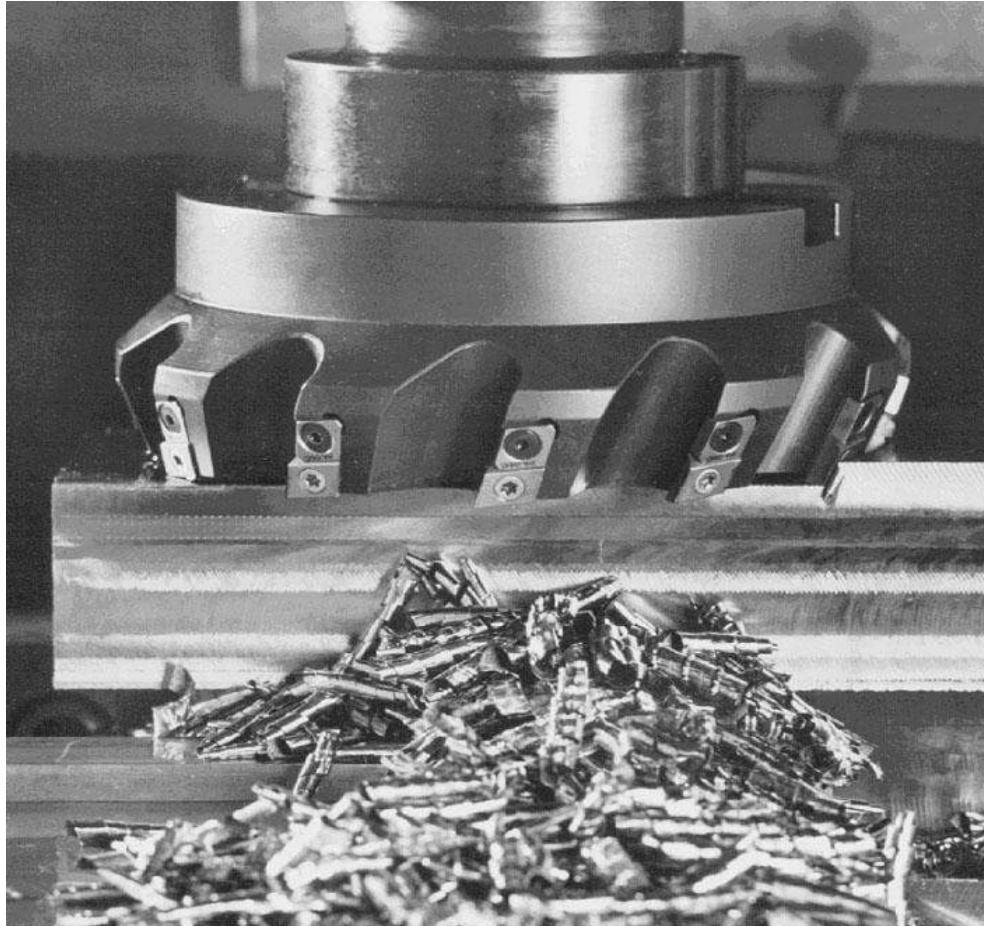
Figure 24.5 A face-milling cutter with index able inserts. Source: Courtesy of Ingersoll Cutting Tool Company.
