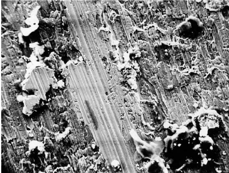
Figure 20.21 Surfaces produced on steel by cutting, as observed with a scanning electron microscope: (a) turned surface and (b) surface produced by shaping. Source: J. T. Black and S. Ramalingam.
