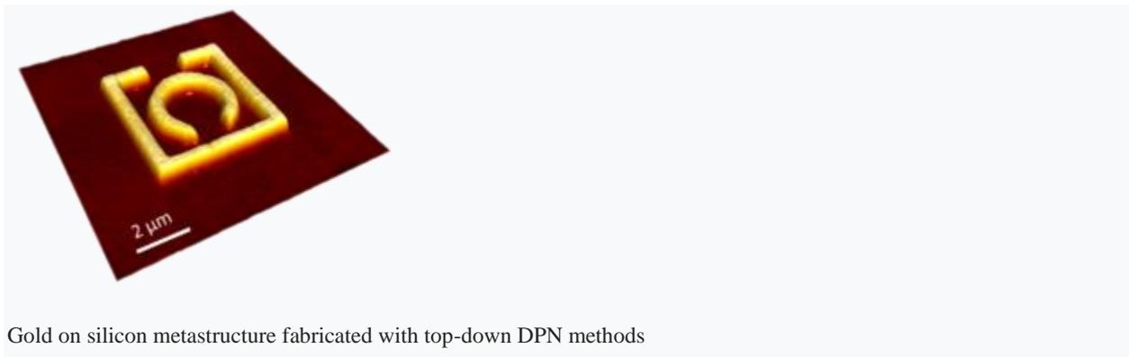
Gold on silicon metastructure fabricated with top-down DPN methods
