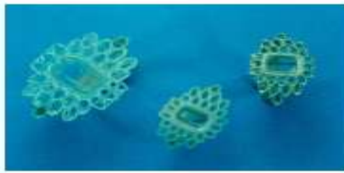
Figure 7.16: An investment cast silver alloy prototype of a brooch (right), the full-scale wax pattern produced from the silicon rubber molding (center), and the two-time scaled SLA model to aid visualization (left)
