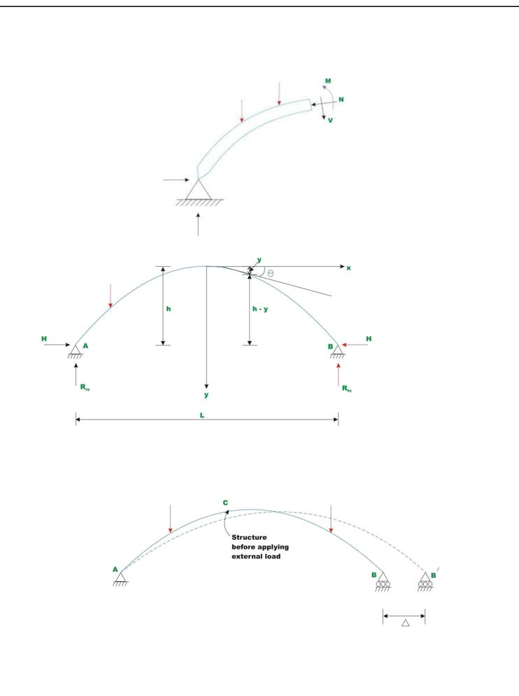
The fourth equation is written considering deformation of the arch. The unknown redundant reaction  $H_b$  is calculated by noting that the horizontal displacement of hinge *B* is zero.
