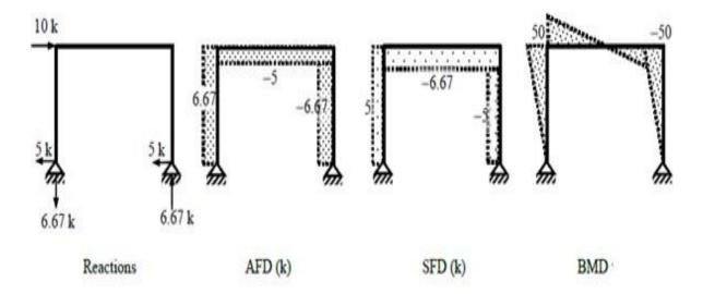
(ii) dosi =  $3 \times 3 + 6 - 3 \times 4 = 3$ Assumption  $1 \Rightarrow H_A = H_D = 10/2 = 5 \text{ k}$ , Assumption  $2 \Rightarrow BM_E = BM_F = 0$   $\therefore BM_F = 0 \Rightarrow H_A \times 5 + M_A = 0 \Rightarrow M_A = -25 \text{ k-ft}$ ; Similarly  $BM_E = 0 \Rightarrow M_D = -25$   $\therefore \sum M_A = 0 \Rightarrow -25 - 25 + 10 \times 10 - V_D \times 15 = 0 \Rightarrow V_D = 3.33 \text{ k}$  $\therefore \sum F_y = 0 \Rightarrow V_A + V_D = 0 \Rightarrow V_A = -3.33 \text{ k}$
