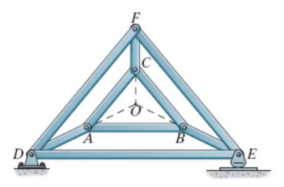
Thus an external load can be applied at A, B or C & cause the truss to rotate slightly
