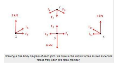
4. Write out the equilibrium equations for each of the joints. You should treat the joints as particles, so there will be force equations but no moment equations. With either two (for 2D problems) or three (for 3D problems) equations for each joint, this should give you a large number of equations.
