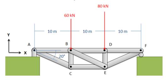
2. Find the force acting in each of the members of the truss shown below. Remember to specify if each member is in tension or compression.
