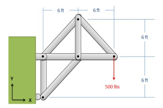
3. Find the force acting in each of the members of the truss shown below. Remember to specify if each member is in tension or compression.
