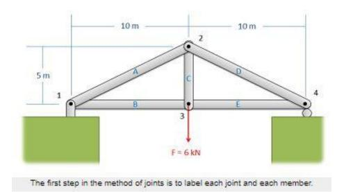
2. Treating the entire truss structure as a rigid body, draw a free body diagram, write out the equilibrium equations, and solve for the external reacting forces acting on the truss structure. This analysis should not differ from the analysis of a single rigid body.
