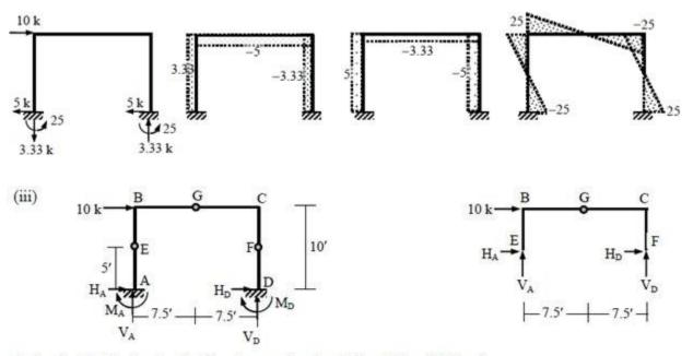
$\begin{array}{l} dosi = 3 \times 4 + 6 - 3 \times 5 - 1 = 2; \ \therefore \ Assumption \ 1 \ and \ 2 \Rightarrow BM_E = BM_F = 0 \\ \therefore BM_E = 0 \ (bottom) \Rightarrow -H_A \times 5 + M_A = 0 \Rightarrow M_A = 5H_A; \ Similarly \ BM_F = 0 \Rightarrow M_D = 5H_D \\ Also \ BM_E = 0 \ (free \ body \ of \ EBCF) \Rightarrow 10 \times 5 - V_D \times 15 = 0 \Rightarrow V_D = 3.33 \ k \\ \therefore \sum F_y = 0 \Rightarrow V_A + V_D = 0 \Rightarrow V_A = -V_D = -3.33 \ k \end{array}$
