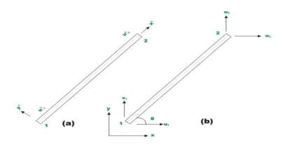
The nodes of the truss member be identified by 1 and 2. Let  $u'_1$  and  $u'_2$  be the displacement of nodes 1 and 2 in local co ordinate system. In global co ordinate system, each node has two degrees of freedom. Thus,  $u_1,v_1$  and  $u_2,v_2$  are the nodal displacements at nodes 1 and 2 respectively along x - and y - directions.
