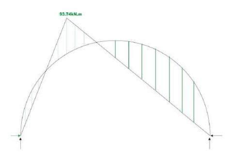
A two hinged parabolic arch of constant cross section has a span of 60m and a rise of 10m. It is subjected to loading as shown . Calculate reactions of the arch if the temperature of the arch is raised by. Assume co-efficient of thermal expansion as
