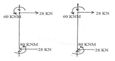
Using F x = 0 for the entire frame R = 28 + 28 = 56 KN
