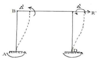
Since both ends are fixed, columns are of same length & I and assuming joints B & C are temporarily restrained from rotating and resulting fixed end moment are assumed.
