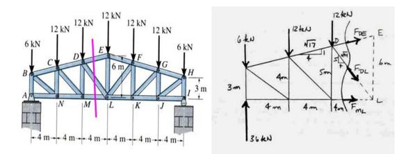
Analyzing the entire truss, we get FX = AX = 0. By symmetry, the vertical support reactions are AY = IY = 36 kN
