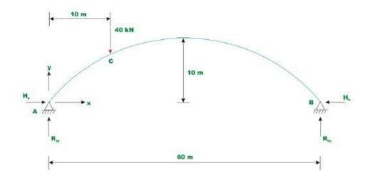
Taking Aas the origin, the equation of two hinged parabolic arch may be written as,
