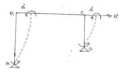
Since ends A & D are hinged and columns AB & CD are of different lengths
