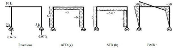
(ii) dosi =  $3 \times 3 + 6 - 3 \times 4 = 3$ Assumption  $1 \Rightarrow H_A = H_D = 10/2 = 5 \text{ k}$ , Assumption  $2 \Rightarrow BM_E = BM_F = 0$   $\therefore BM_F = 0 \Rightarrow H_A \times 5 + M_A = 0 \Rightarrow M_A = -25 \text{ k-ft}$ ; Similarly  $BM_E = 0 \Rightarrow M_D = -25$   $\therefore \sum M_A = 0 \Rightarrow -25 - 25 + 10 \times 10 - V_D \times 15 = 0 \Rightarrow V_D = 3.33 \text{ k}$  $\therefore \sum F_y = 0 \Rightarrow V_A + V_D = 0 \Rightarrow V_A = -3.33 \text{ k}$
