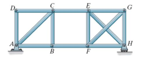
To determine the internal stability of a compound truss, it is necessary to identify the way in which the simple truss are connected together
