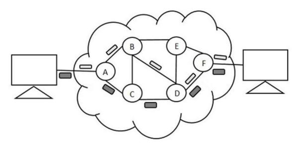
In this technique, the data is stored and forwarded. The technique is also called the **Store-and-Forward** technique. This technique was considered a substitute to circuit switching. But the transmission delay that followed the end to end delay of message transmission added to the propagation delay and slowed down the entire process.
