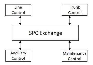
The processors used by SPC are designed based on the requirements of the exchange. The processors are duplicated; and, using more than one processor makes the process reliable. A separate processor is used for the maintenance of the switching system.
