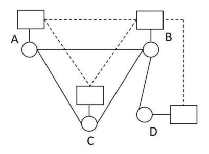
The signaling paths for the speech paths A-B, A-C-B and B-D are A-B, A-C-B and B-D respectively. The advantages of this signaling are:
