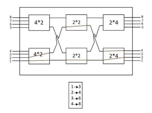
In the above figure, where there are 4 inputs and 2 outputs, the Subscriber 1 was connected to Line 3 and the Subscriber 2 was connected to Line 4. The red-colored lines indicate the connections. However, there will be more requests coming; a calling request from subscriber 3 and subscriber 4 if made cannot be processed, as the call cannot be established.
