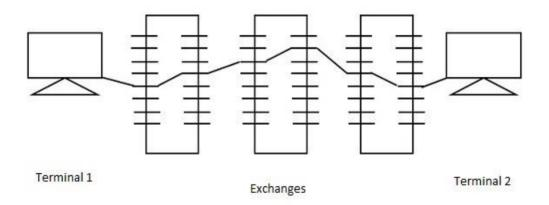
Time division switches use time division multiplexing, in switching. The two popular methods of TDM are TSI (Time and Slot Interchange) and TDM bus. The data sent at the
