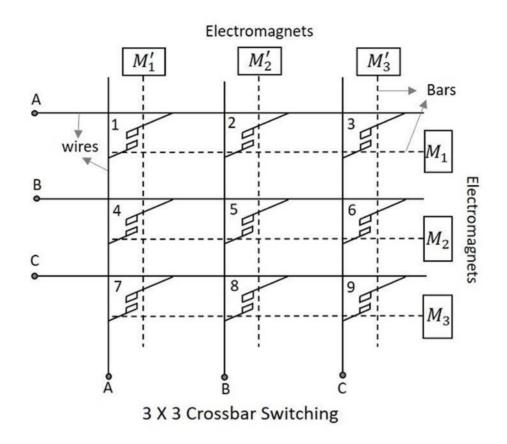
The Crossbar matrix contains an array of horizontal and vertical wires shown by solid lines in the following figure, which are both connected to initially separated contact points of switches. The horizontal and vertical bars shown in dotted lines in the above figure are mechanically connected to these contact points and attached to the electromagnets.
