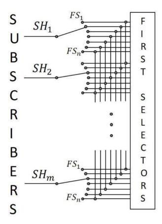
When a calling subscriber lifts the handset to make a call, the selector hunter activates the interrupter mechanism, which steps up the wiper until a free first group selector is found at the outlet. One of the bank contacts of the selector hunter, at this point, senses whether the first group selector is free or busy. Once a free first selector is sensed, the interrupter is disabled and the connection is established, where the first selector sends out a dialer tone to the calling subscriber.
