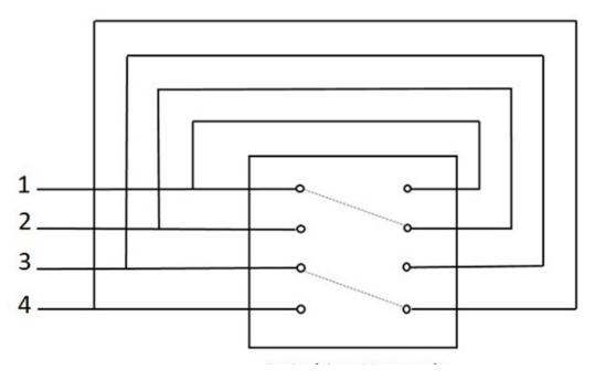
As one connection can be given to one line per time, only N/2 connections are established for N inlets of a folded network. Such a network can be called as **Non-blocking network**. In a non-
