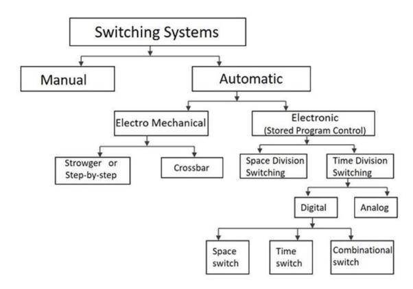
The switching systems in the early stages were operated **manually**. The connections were made by the operators at the telephone exchanges in order to establish a connection. To minimize the disadvantages of manual operation, automatic switching systems were introduced.
