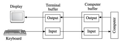
(a) Independent buffers for input and output: asynchronous mode
