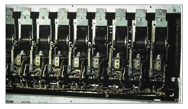
Thus, the wiper assembly establishes the call; after completion of which it comes back to the home position. For this purpose, the rotary magnet is operated by the current and thus the wiper assembly moves through the remaining contacts of the level. A restoring spring forces the wiper assembly to drop vertically and then return horizontally to the home position.
