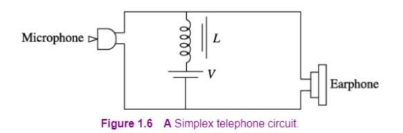
elements of the telephone communication system. Microphone converts speech signals into electrical signals and the earphone converts electrical signals into audio signals. Most commonly used microphone is a carbon microphone. Carbon microphones do not produce high fidelity signals but give out strong electrical signals at acceptable quality levels for telephone conversation.
