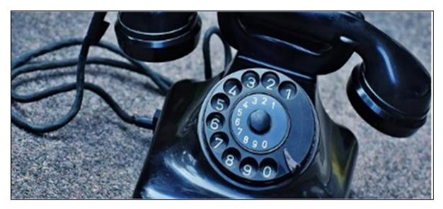
The dial is operated by placing the finger in the hole appropriate to the digit to be dialed. Now, drawing the fingerplate round in the clockwise direction to the finger stop position and letting the dial free by withdrawing the finger, makes a number dialed. The fingerplate and the associated mechanism now return to the rest position under the influence of a spring. The dial is ready for the next number.
