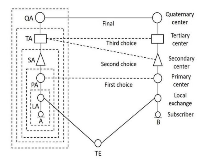
To decide the routing on a particular connection, the following three methods are used:
