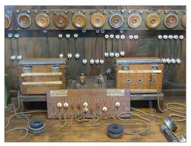
The above figure shows an early model of the PBX system. The PBX is usually operated and owned by the local office where the users are connected through it within that limited area.
