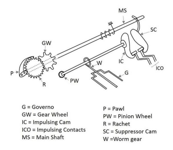
The suppressor cam helps in keeping the Impulsing cam away from the Impulsing contacts. When the rotary dial is in rest position, then the Impulsing contacts are away from the Impulsing cam. When a number is dialed, by placing the finger in the dial hole, which means the dial is displaced from its position, then the Impulsing contacts come near the Impulsing cam. This rotation of the finger plate, causes the rotation of the Main shaft.
