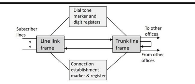
The call processing in a Crossbar exchange is done in three stages, named as Pre-Selection, Group Selection and Line Selection.
