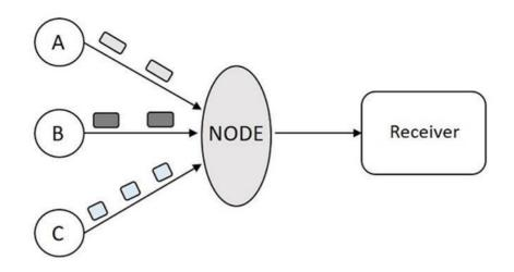
In the above figure, when the data packets arrive at Node from the senders A, B and C then the node cannot transmit the data to the receiver at a faster rate. There occurs a delay in transmission or may be data loss due to heavy congestion.
