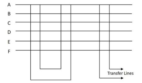
The switch shown in the above figure is blocking both internally and externally with two simultaneous internal and two simultaneous external calls. The number of Crosspoint switches in this case is N(2K+L), where N is the number of subscribers, L is the number of transfer lines and K is the number of simultaneous calls that can be supported locally.
