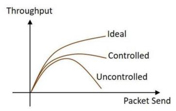
The techniques used for congestion control are of two types – open loop and closed loop. The loops differ by the protocols they issue.
