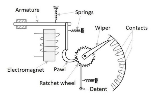
When the input voltage energizes the Electromagnet, the armature is pulled down towards the magnet. Now as the armature gets attracted towards the electromagnet, the pawl falls one position down the previous one in the ratchet wheel. The detent prevents the movement of the ratchet wheel.
