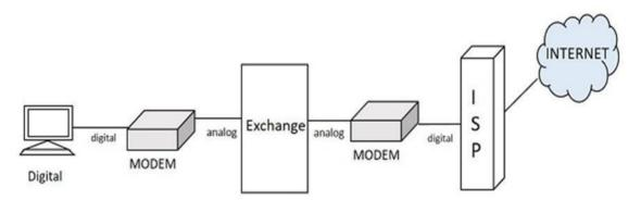
The above figure shows that the digital signals have to be converted into analog and analog signals to digital using modem during the whole path. What if the digital information at one end reaches to the other end in the same mode, without all these connections? It is this basic idea that lead to the development of **ISDN**.
