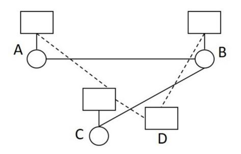
The signaling paths for the speech paths A-B and B-C are A-C-D-B and B-D-C respectively. The network topologies are different for signaling and speech networks. Though this scheme offers flexibility as there is no switching center, it is a bit complex, as the signal messages may be transferred between the two end switching systems via any available path in the common channel signaling network according to its own routing principles.
