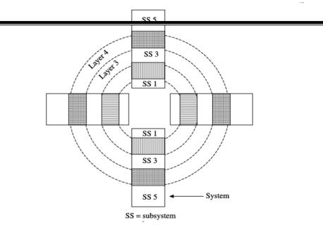
Systems, subsystems and layers in ISO-OSI model.
