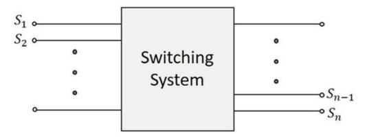
With the introduction of switching systems, the need for traditional connections between the subscribers reduced. All the subscribers need to have a connection with the switching system, which makes or breaks any connection, requested by the calling subscriber. The switching system, which is also called the **Telephone Exchange**, takes care of establishing the calls. Hence, the total number of such links is equal to the number of subscribers connected to the system.
