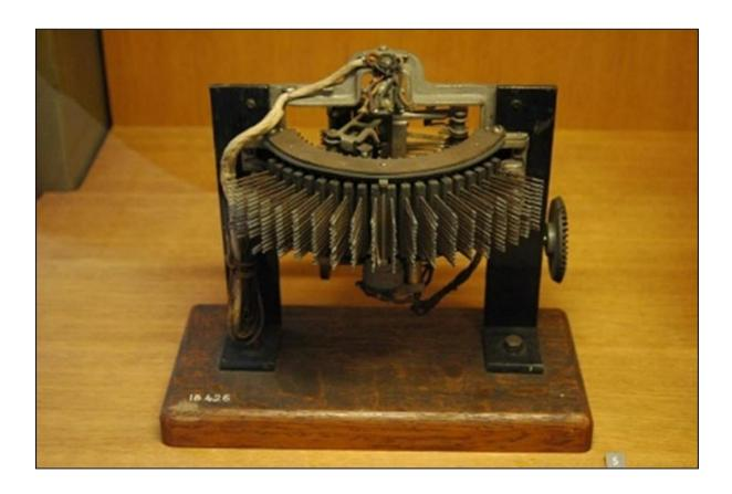
The type of switching mechanism discussed here is known as the **reverse drive type** because, here the ratchet wheel moves when the armature return to its rest position. If it is arranged such that the wheel moves during the forward motion of the armature it is known as the **forward drive type**. The Reverse drive type mechanism is prevalent in uni- selectors and the forward drive type mechanism in the two-motion selectors.
