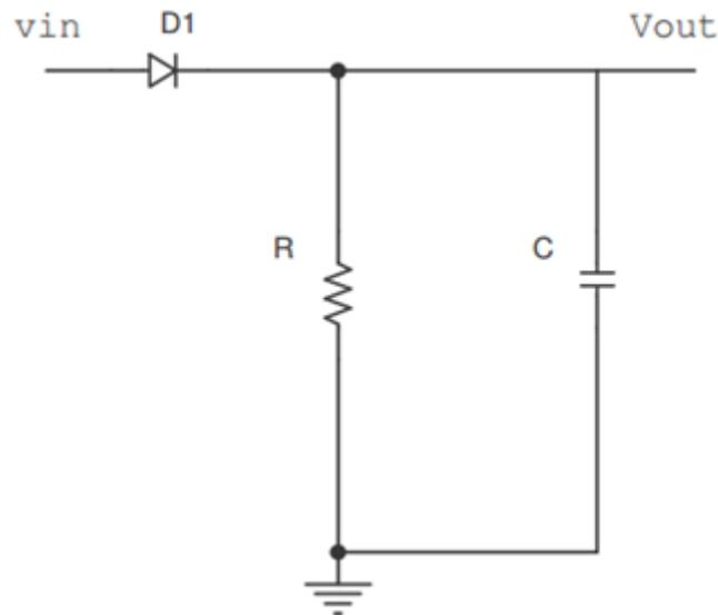
Figure 3.6: Envelop Detector
