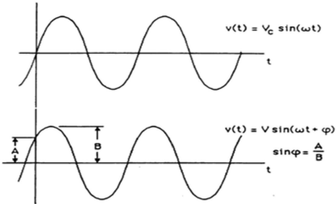
Figure C.4: Phase measurement
