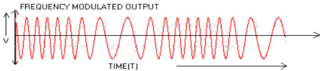
Figure 5.5: Frequency Modulated Waveform
