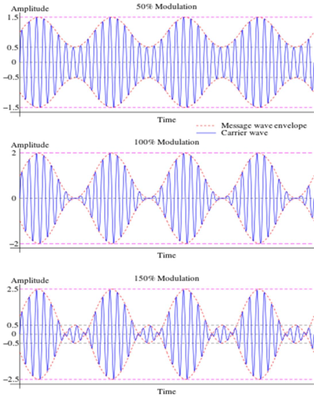
Figure 3.9: Types of Amplitude Modulated Wave Forms
