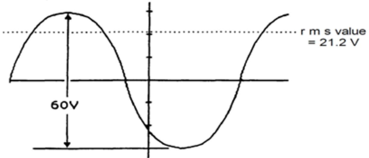
Figure C.2: Sinusoidal waveform
