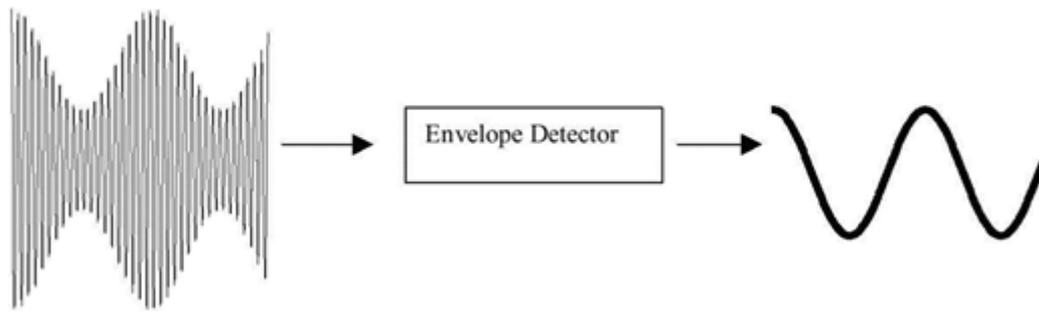
Figure 3.5: Demodulation of an AM Signal
