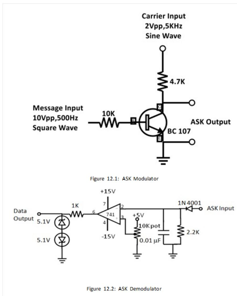
Figure 16.1: Modulator and Demodulator
