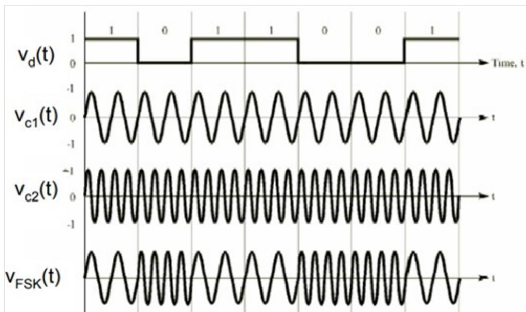
Figure 13.2: Simulation Result
