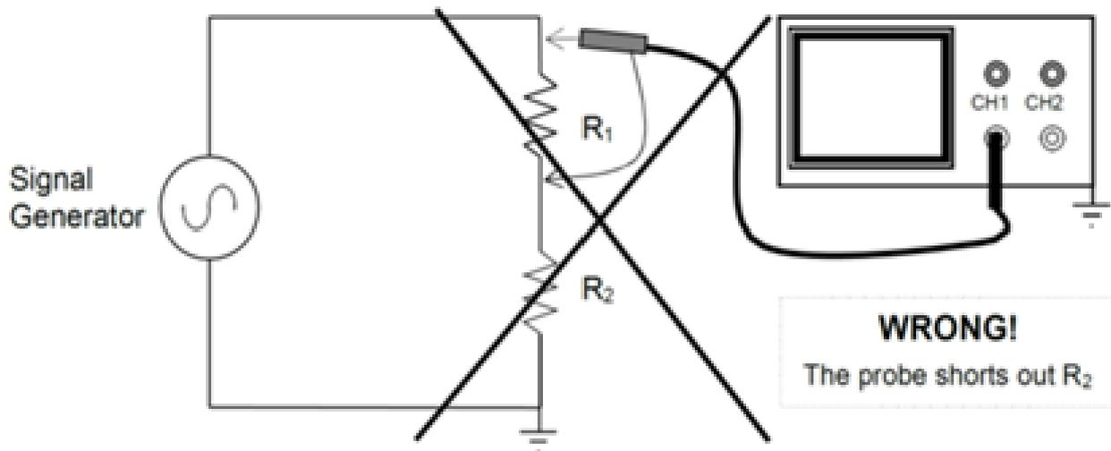
Figure C.1: Grounding error
