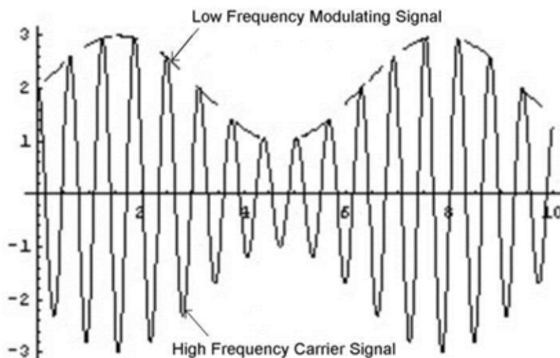
Figure 3.3: Amplitude Modulated Waveform
