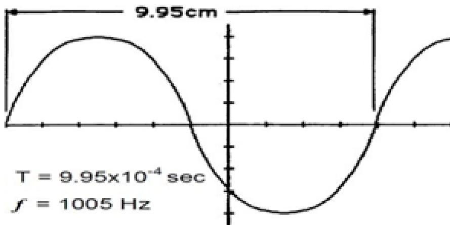
Figure C.3: Frequency measurement
