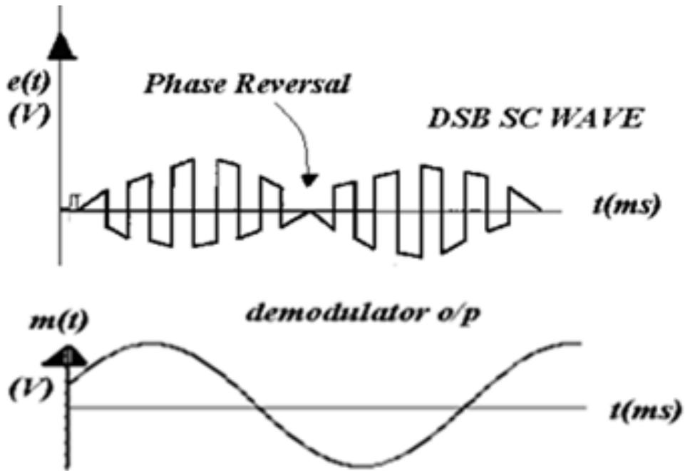
Figure 4.4: DSBSC Modulated and Demodulated Waveforms
