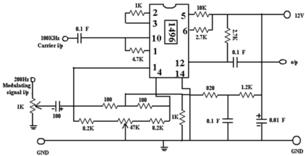
Figure 4.1: Balance Modulator
