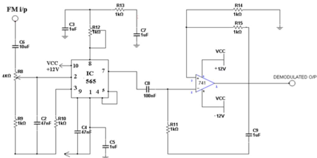
Figure 5.2: Frequency De Modulator
