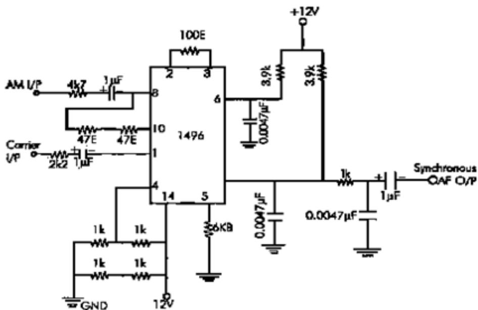
Figure 4.2: Synchronous De-Modulator
