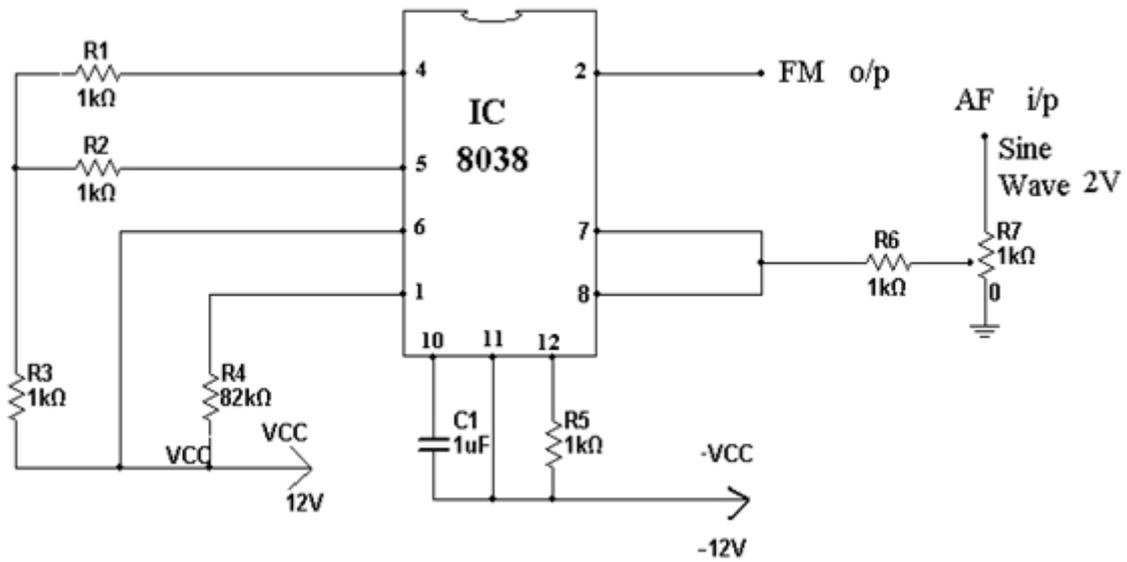
Figure 5.1: Frequency Modulator
