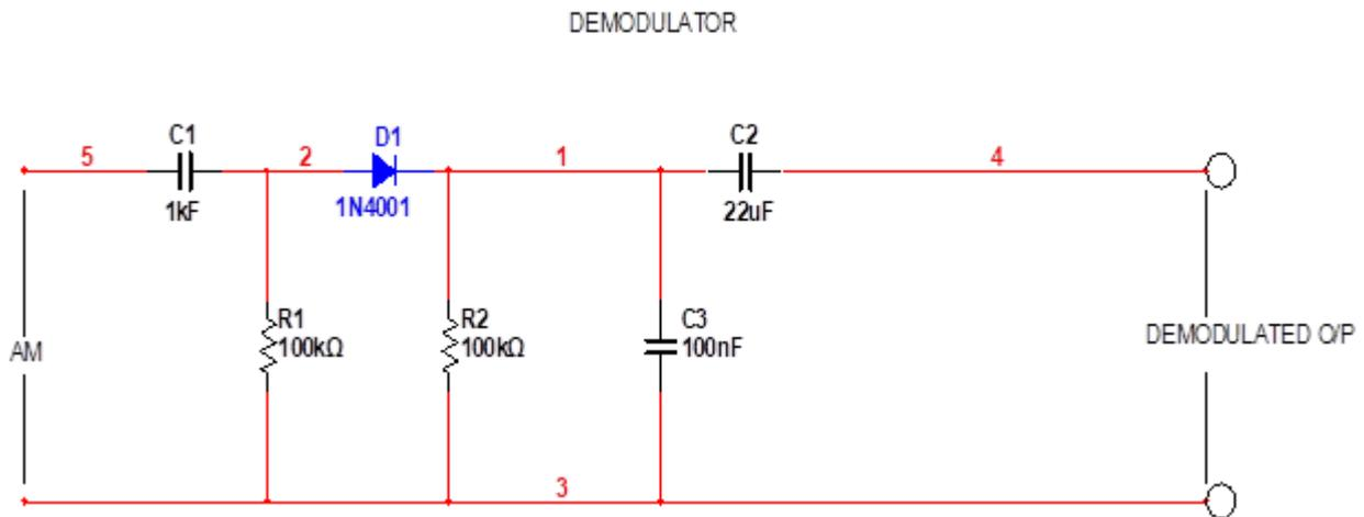
Figure 3.2: Amplitude De-Modulator
