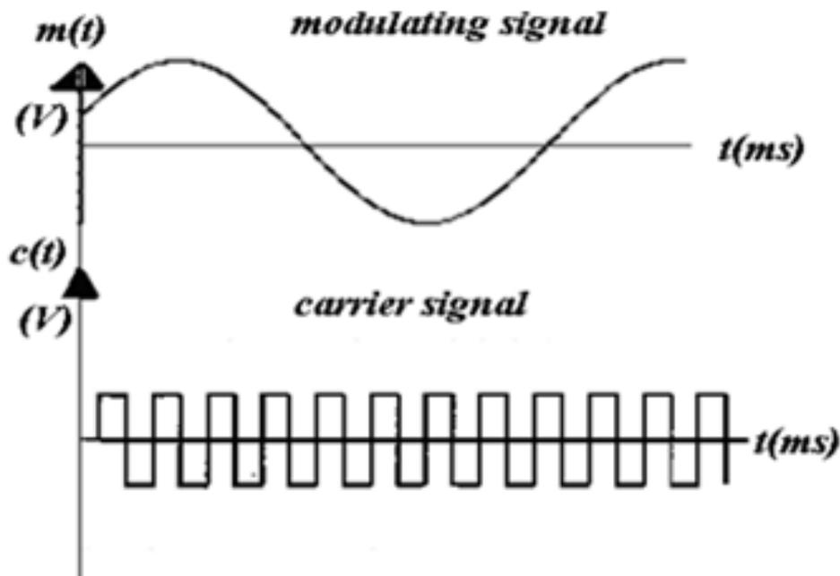
Figure 4.3: Message And Carrier Waveforms
