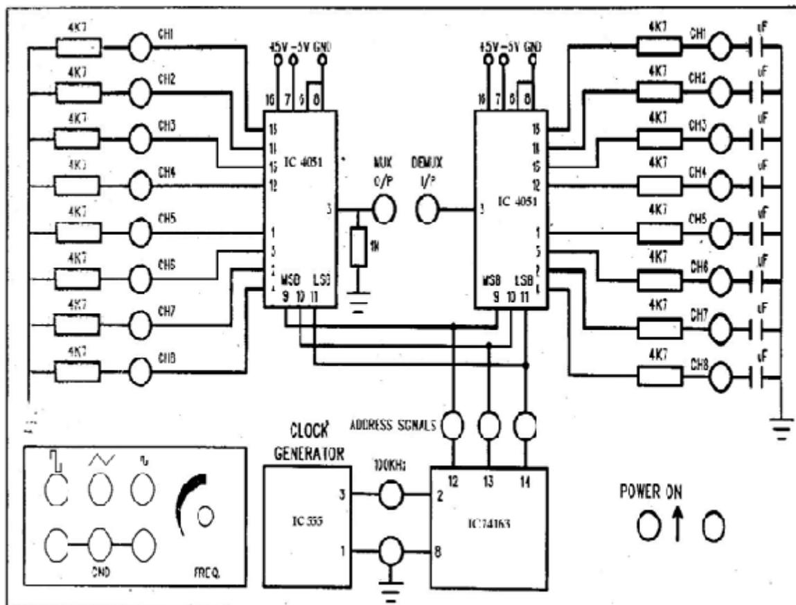
Figure 12.1: Time Division Multiplexing And De Multiplexing Circuit
