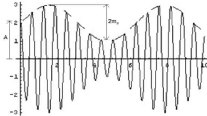
Figure 3.4: AM Modulated Signal Showing Values
