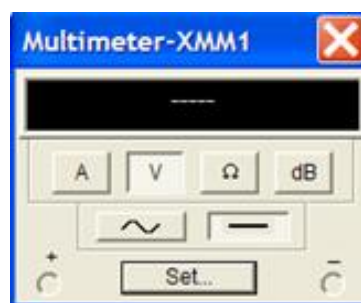
Figure 18.9: Selection of voltmeter in multimeter
