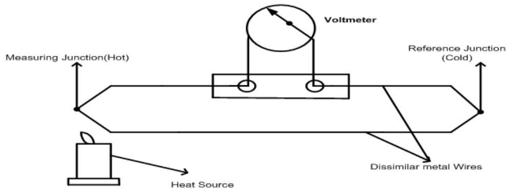
Figure 2.1: Thermocouple.
