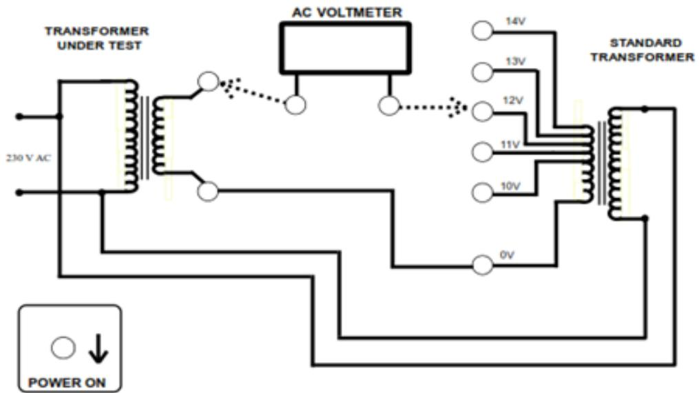
Figure 8.1: Turns Ratio Diagram.
