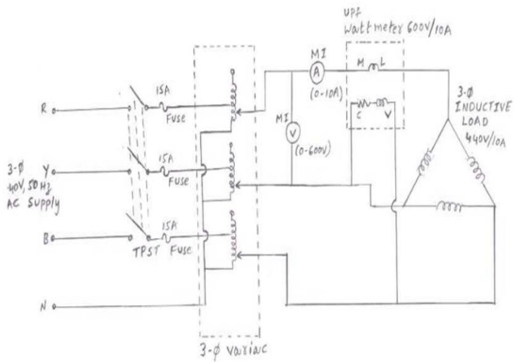
Figure 9.1: Circuit Diagram of Measurement of 3-Phase Reactive Power using Single Wattmeter.
