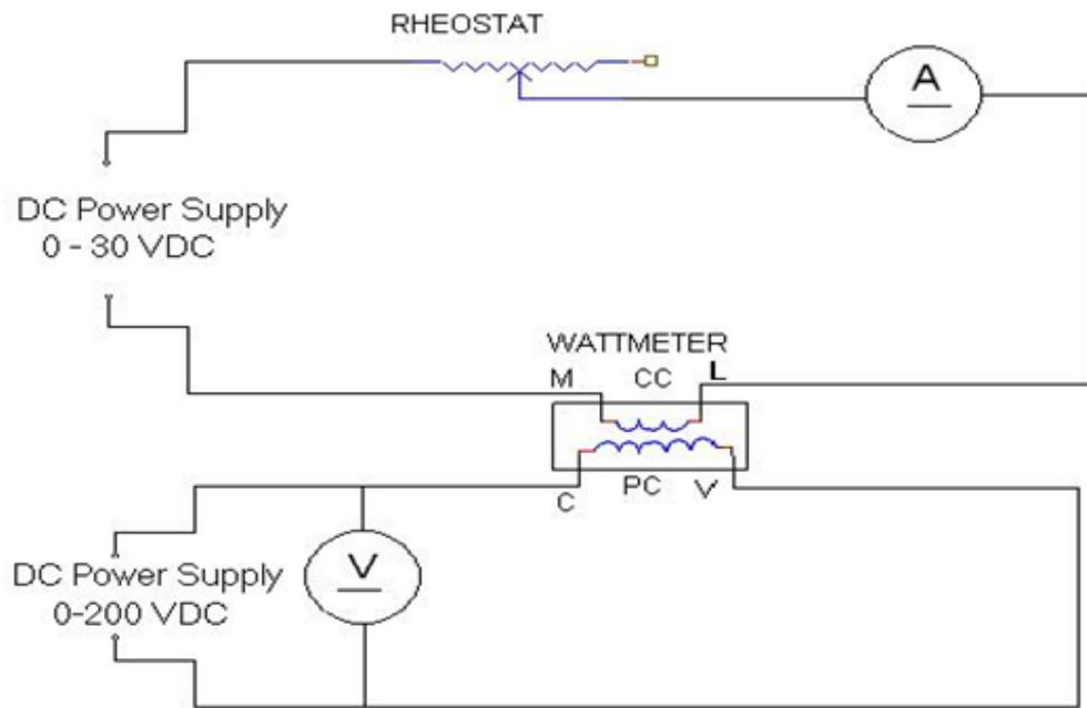
Figure 6.1: Calibration of LPF Wattmeter by Phantom Testing.
