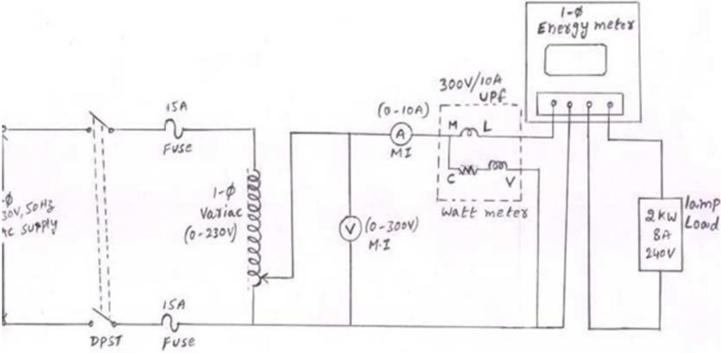
Figure 7.1: Calibrations and Testing of Single Phase Energy Metere.
