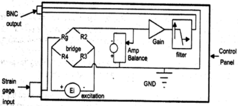
Figure 4.4: Circuit Diagram of Resistance Strain Gauge Strain .
