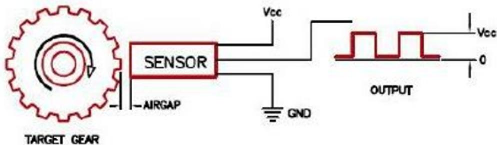
Figure 2.4: Magnetic pickup (Proximity) sensor.
