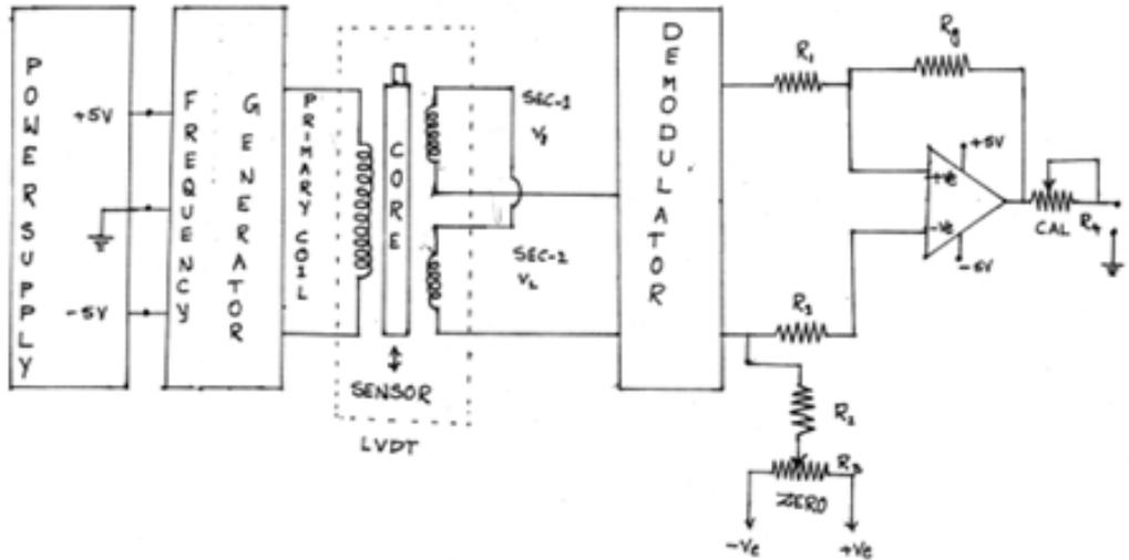
Figure 5.1: Circuit Diagram of LVDT and Capacitance Pickup – Characteristics and Calibration.
