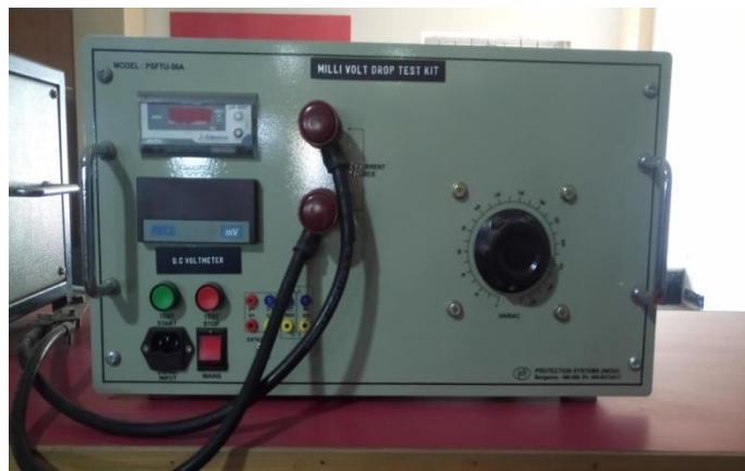
Fig 2.1. Milli-volt drop setup
