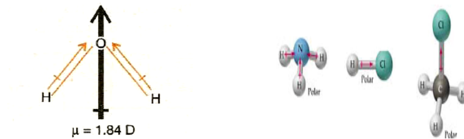
Fig. Polar molecules with net dipole moment ( \mu \neq 0 )
