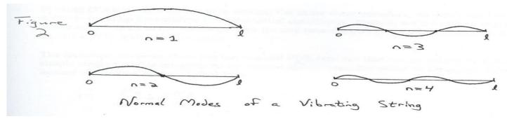
Thus suppose a string of length I, and string mass per unit length  $\delta$ , is tightened so that the values of T, the string tension, along the other constants make the value of  $\lambda_1 = \frac{\sqrt{T}}{2I\sqrt{\delta}}$  equal to 440. Then if the string is made to vibrate by striking or plucking it, then its fundamental (lowest) tone would be the A above middle C.
