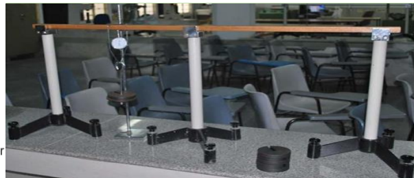
fig.12.2: Setup of Continuous beam deflection
