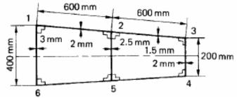
8. a) Draw the neat sketches of idealized simple wing section. Derive bending stress and shear flow [7M] distribution.
