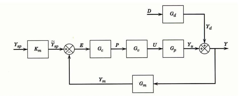
Standard block diagram of a feedback control system
