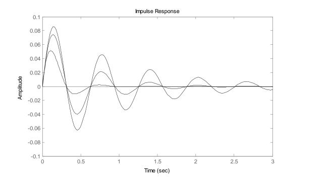
$$h(t) = \frac{\sigma^2 + \omega^2}{\omega} e^{-\sigma t} \sin(\omega t) \ 1(t)$$
