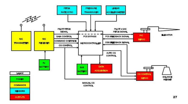
Displacement (Position) feedback as a tool in SAS
