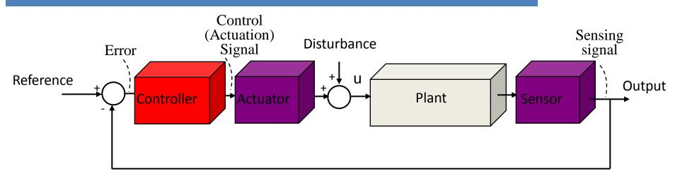
Error signal= Reference – Sensing signal
