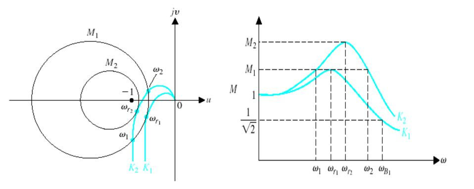
Polar plot of  $G(j\omega)$  for two values of a gain  $(K_2 > K_1)$ .
