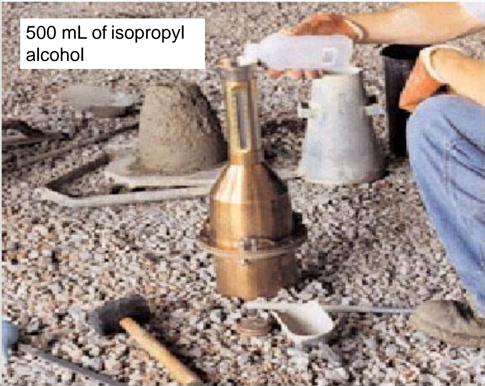
Fig. 16-6. Volumetric air meter. (69886)
