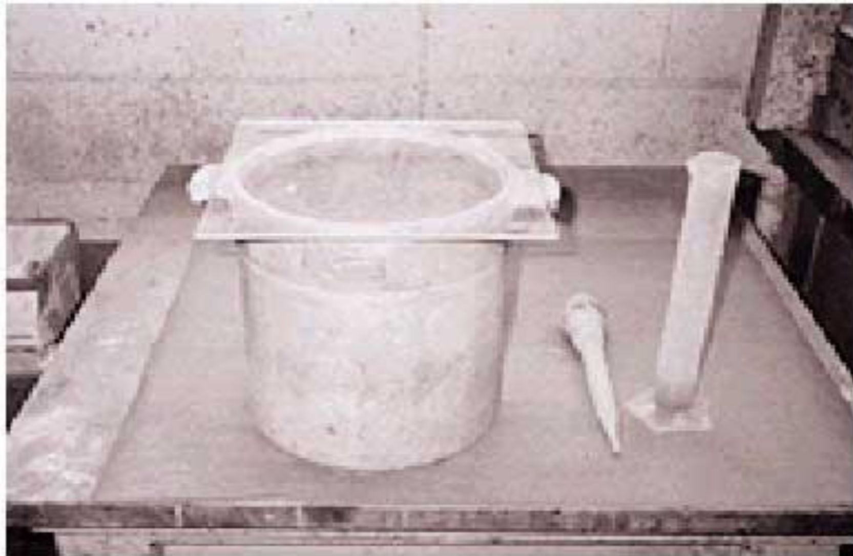
Fig. 16-12. ASTM C 232 test for bleeding of concrete; Method A without vibration. The container has an inside diameter of about 255 mm and height of about 280 mm. The container is filled to a height of about 255 mm and covered to prevent evaporation of the bleed water. (69780)
