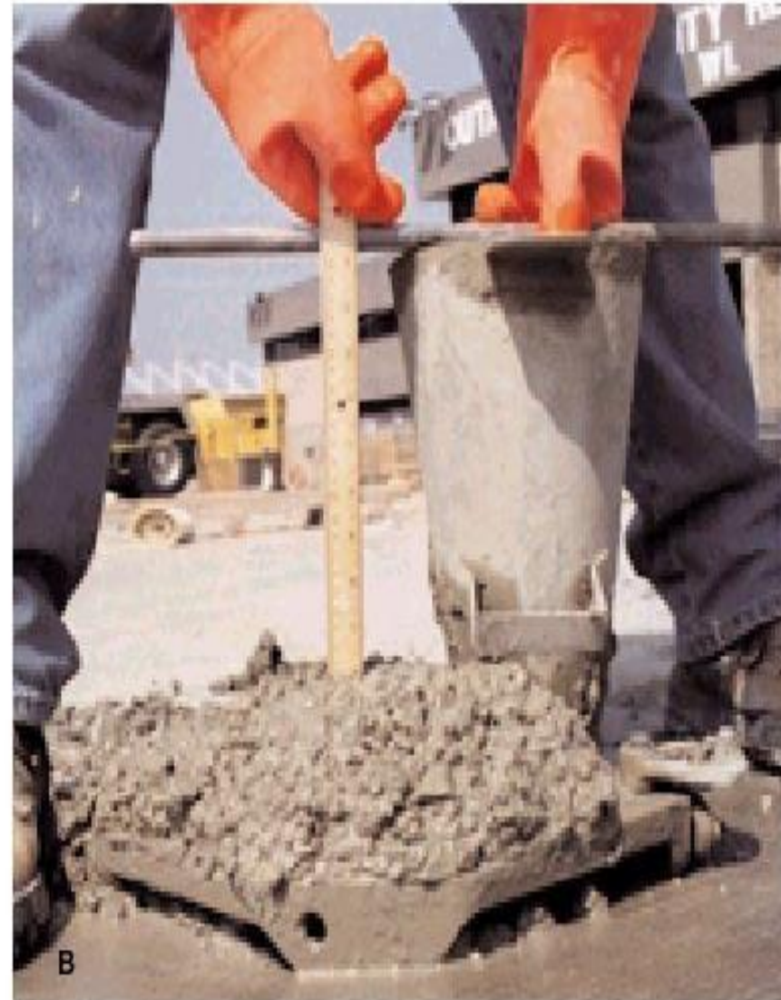
Fig. 16-2. Slump test for consistency of concrete. Figure A illustrates a lower slump, Figure B a higher slump. (69786, 69787)
