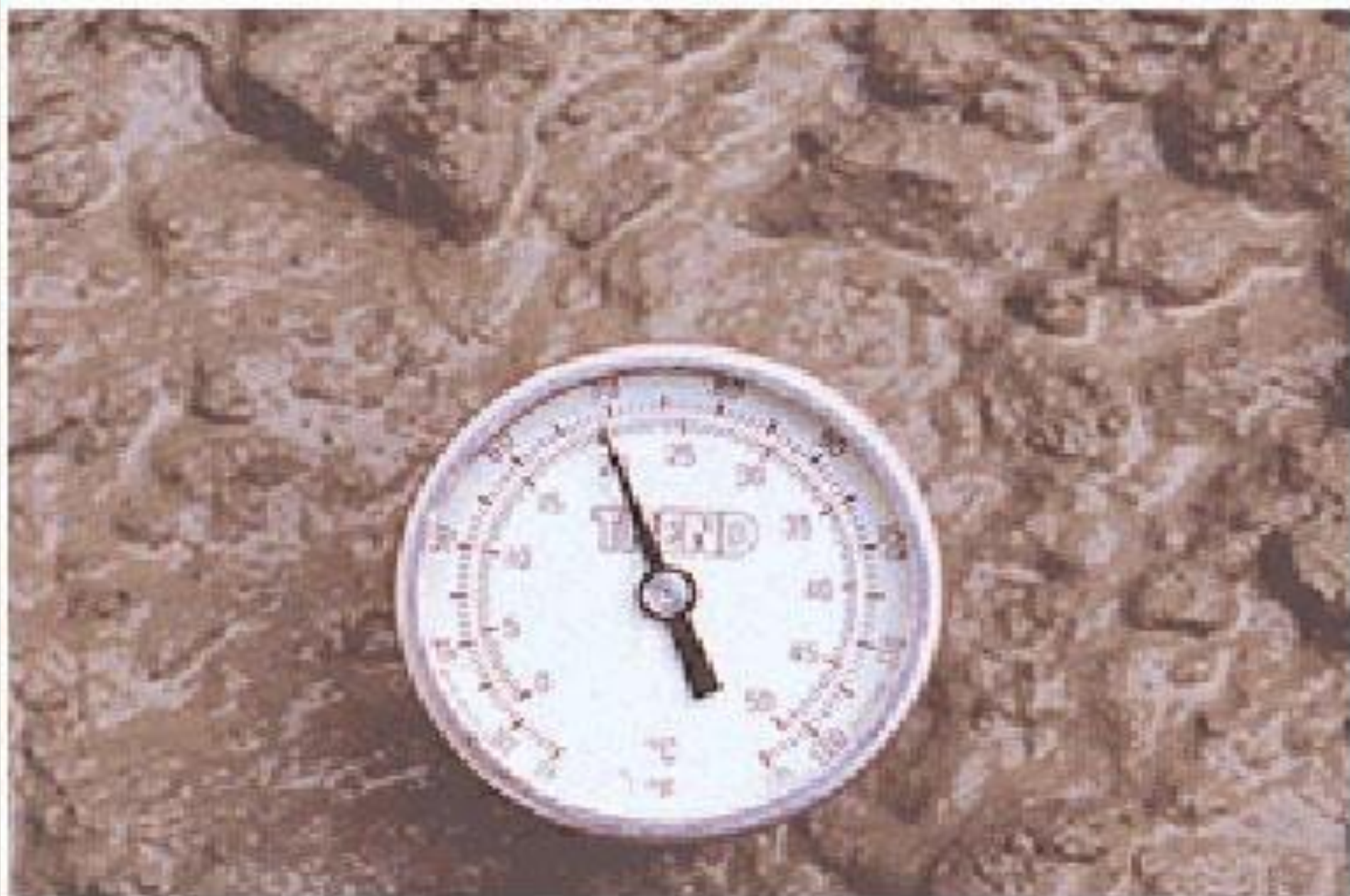
Fig. 16-3. A thermometer is used to take the temperature of fresh concrete. (69885A)
