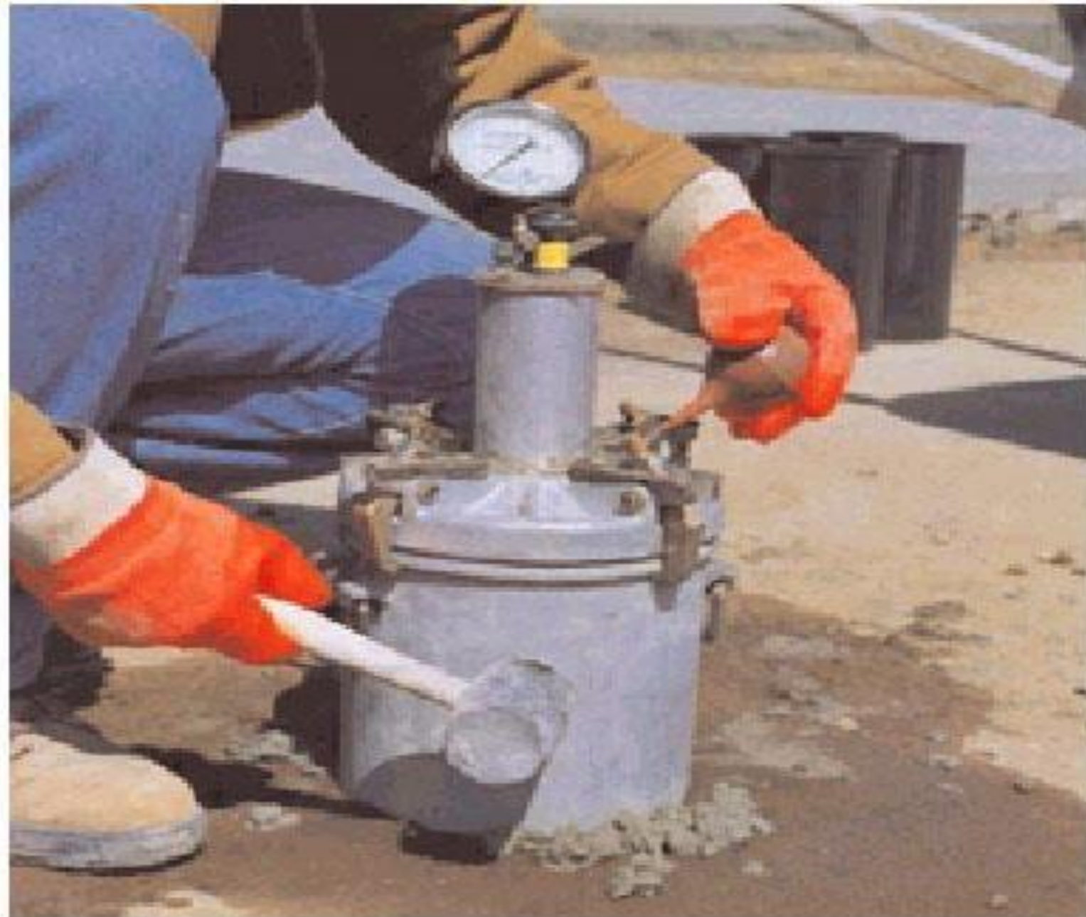
Fig. 16-5. Pressure-type meter for determining air content. (69766)
