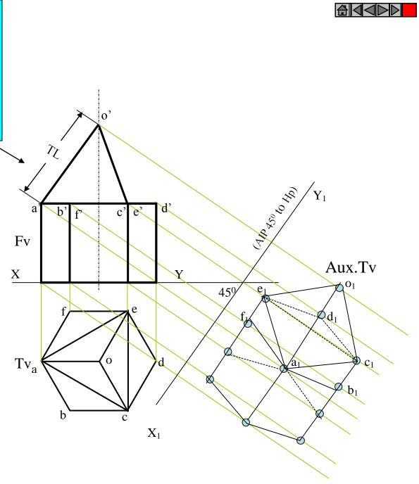
Problem 12: A frustum of regular hexagonal pyrami is standing on it's larger baseOn Hp with one base side perpendicular to Vp.Draw it's Fv & Tv.Project it's Aux.Tv on an AIP parallel to one of the slant edges showing TL.Base side is 50 mm long , top side is 30 mm long and 50 mm is height of frustum.
