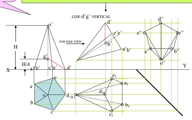
*IMPORTANT:* When a solid is freely suspended from a corner, then line joining point of contact & C.G. remains vertical. (Here axis shows inclination with Hp.) So in all such cases, assume solid standing on Hp initially.)
