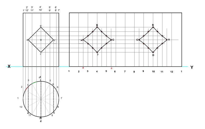
Q.15.21: A frustum of square pyramid has its base 50 mm side, top 25 mm side and axis 75 mm. Draw the development of its lateral surface. Also draw the projections of the frustum (when its axis is vertical and a side of its base is parallel to the VP), showing the line joining the mid point of a top edge of one face with the mid point of the bottom edge of the opposite face, by the shortest distance.
