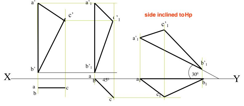
Surface // to Vp Surface inclined to Vp
