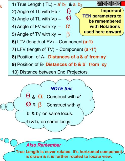
Views are always rotated, made horizontal & further extended to locate TL,  $\theta \& \phi$
