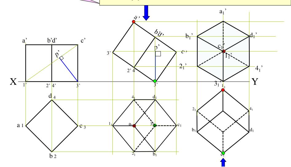
**Problem 6:**A tetrahedron of 50 mm long edges is resting on one edge on Hp while one triangular face containing this edge is vertical and 45<sup>o</sup> inclined to Vp. Draw projections.
