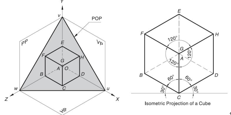
Isometric projection is often constructed using isometric scale which gives dimensions smaller than the true dimensions.
