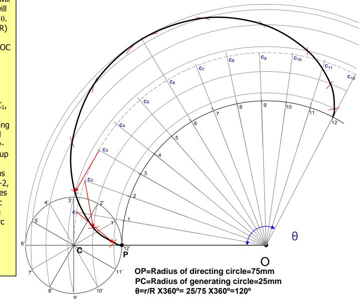
**PROBLEM 26:** DRAW LOCUS OF A POINT ON THE PERIPHERY OF A CIRCLE WHICH ROLLS FROM THE INSIDE OF A CURVED PATH. **Take diameter of rolling circle 50 mm and radius of directing circle (curved path) 75 mm.**
