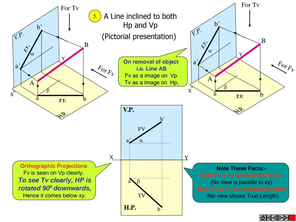
**Orthographic Projections** Means Fy & Ty of Line AB are shown below, with their apparent Inclinations α&β
