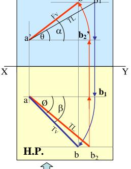
Here a'b<sub>1</sub>' is component of TL ab<sub>1</sub> gives length of FV. Hence it is brought Up to Locus of a' and further rotated to get point b'. a' b' will be Fv. Similarly drawing component of other TL(a'b<sub>1</sub>') TV can be drawn. The most important diagram showing graphical relations among all important parameters of this topic. Study and memorize it as a *CIRCUIT DIAGRAM* And use in solving various problems.
