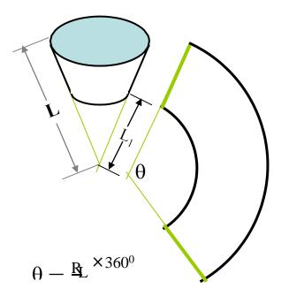
R= Base circle radius of cone L= Slant height of cone  $L_1$  = Slant height of cut part.
