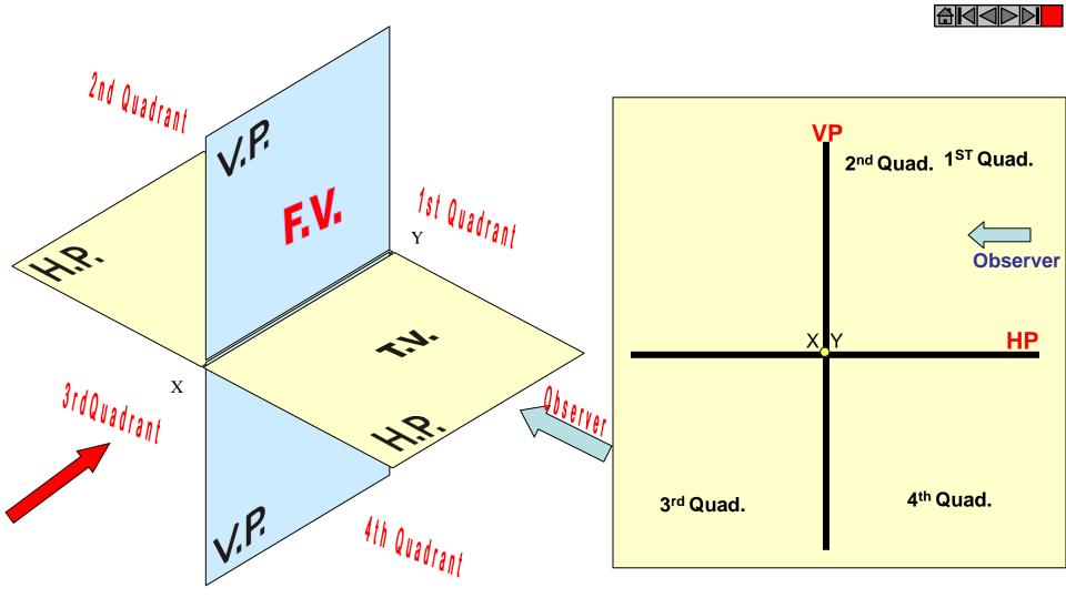
THIS QUADRANT PATTERN, IF OBSERVED ALONG X-Y LINE (IN RED ARROW DIRECTION) WILL EXACTLY APPEAR AS SHOWN ON RIGHT SIDE AND HENCE, IT IS FURTHER USED TO UNDERSTAND ILLUSTRATION PROPERLLY.
