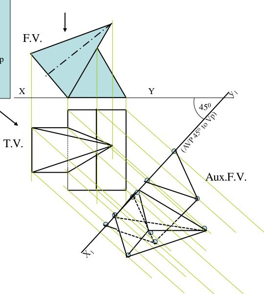
**Problem 11:** A hexagonal prism of base side 30 mm longand axis 40 mm long, is standing on Hp on it's base with one base edge // to Vp. A tetrahedron is placed centrally on the top of it.The base of tetrahedron is a triangle formed by joining alternate corners of top of prism..Draw projections of both solids. Project an auxiliary Tv on AIP 45<sup>o</sup> inclined to Hp.
