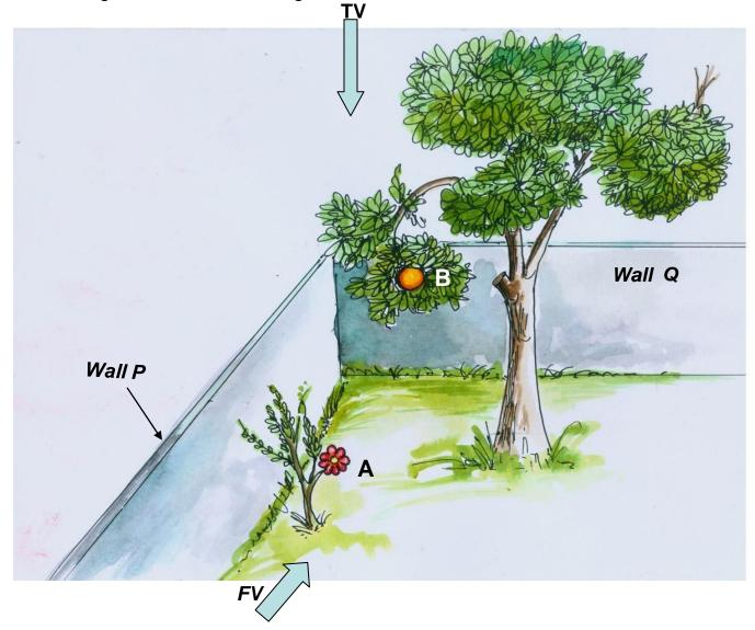
**PROBLEM 15 :-** Two mangos on a tree A & B are 1.5 m and 3.00 m above ground and those are 1.2 m & 1.5 m from a 0.3 m thick wall but on opposite sides of it. If the distance measured between them along the ground and parallel to wall is 2.6 m, Then find real distance between them by drawing their projections.
