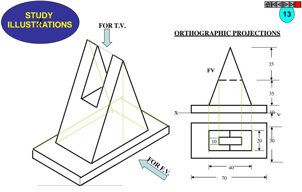
**PICTORIAL PRÉSENTATION IS GIVEN** DRAW FV AND TV OF THIS OBJECT BY FIRST ANGLE PROJECTION METHOD TV
