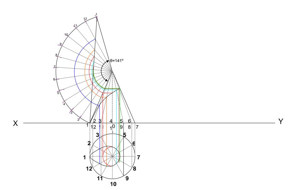
Q.15.11: A right circular cylinder, base 50 mm diameter and axis 60 mm long, is standing on HP on its base. It has a square hole of size 25 in it. The axis of the hole bisects the axis of the cylinder and is perpendicular to the VP. The faces of the square hole are equally inclined with the HP. Draw its projections and develop lateral surface of the cylinder.
