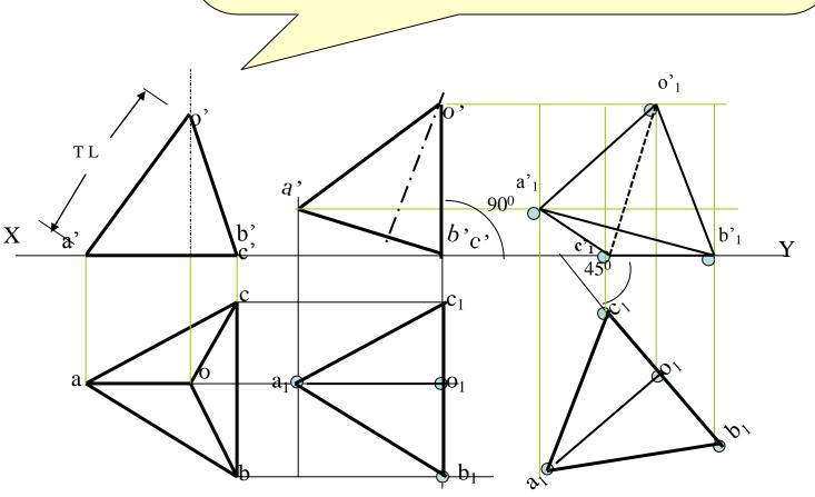
**Problem 1.** A square pyramid, 40 mm base sides and axis 60 mm long, has a triangular face on the ground and the vertical plane containing the axis makes an angle of 45<sup>o</sup> with the VP. Draw its projections. Take apex nearer to VP
