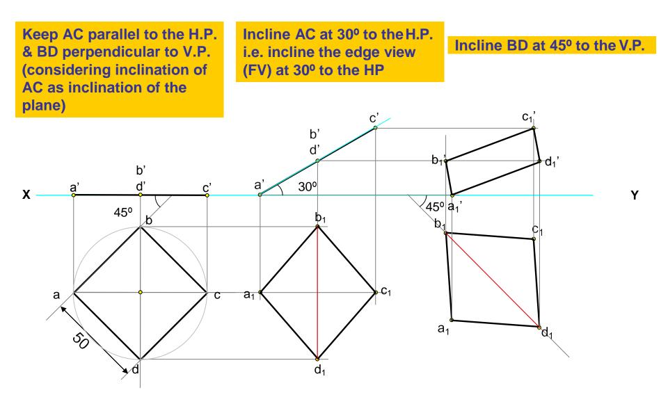
Q: Draw a rhombus of 100 mm and 60 mm long diagonals with longer diagonal horizontal. The figure is the top view of a square having 100 mm long diagonals. Draw its front view.
