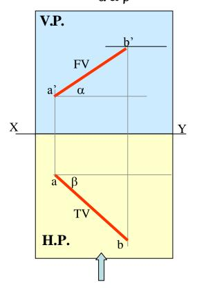
Here TV (ab) is not // to XY line Hence it's corresponding FV a' b' is not showing True Length & True Inclination with Hp.
