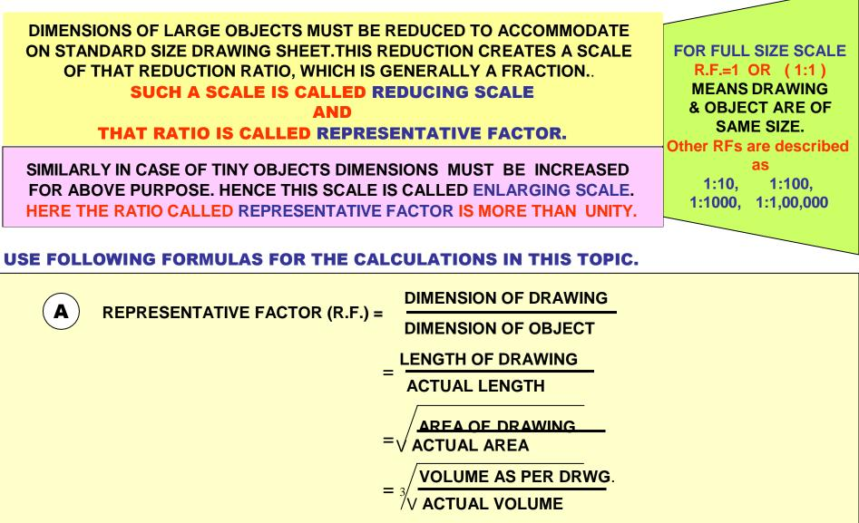
LENGTH OF SCALE = R.F. X MAX. LENGTH TO BE MEASURED.
