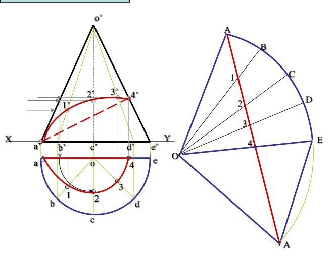
Concept: A string woundd from a point up to the same Point, of shortest length Must appear st. line on it's s Development. Solution steps: Hence draw development, Name it as usual and join A to A This is shortest Length of that string. Further steps are as usual. On dev. Name the points of Intersections of this line with Different generators.Bring Those on Fv & Tv and join by smooth curves. Draw 4' a' part of string dotted As it is on back side of cone.
