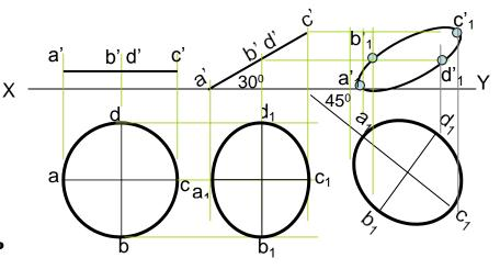
The difference in these two problems is in step 3 only. In problem no.8 inclination of Tv of that AC is given, lt could be drawn directly as shown in  $3^{rd}$  step. While in no.9 angle of AC itself i.e. it's TL, is given. Hence here angle of TL is taken, locus of  $c_1$ Is drawn and then LTV I.e.  $a_1 c_1$  is marked and final TV was completed. Study illustration carefully.
