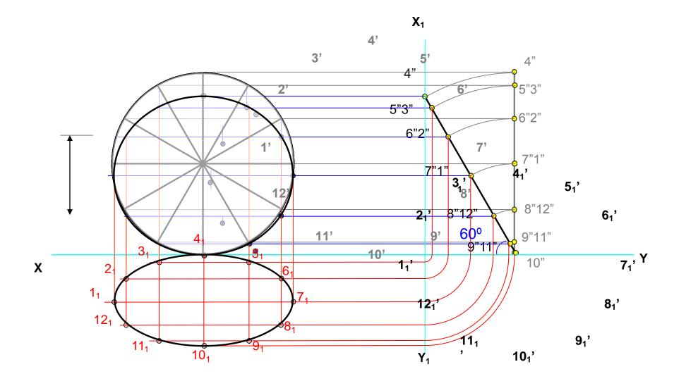
The top view of a plate, the surface of which is inclined at 60° to the HP is a circle of 60 mm diameter. Draw its three views.
