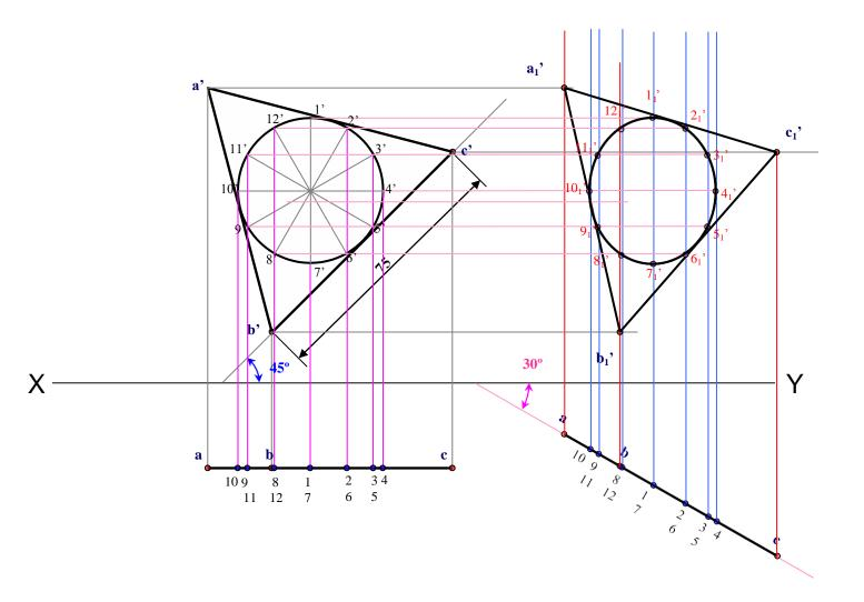
Q12.7: Draw the projections of a regular hexagon of 25mm sides, having one of its side in the H.P. and inclined at 60 to the V.P. and its surface making an angle of 45° with the H.P.
