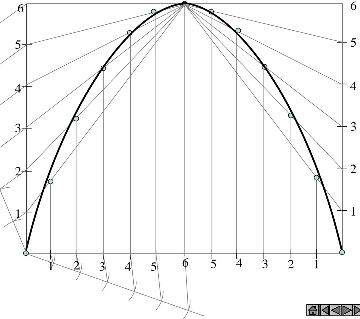
Draw a parabola by tangent method given base 7.5m and axis 4.5m
