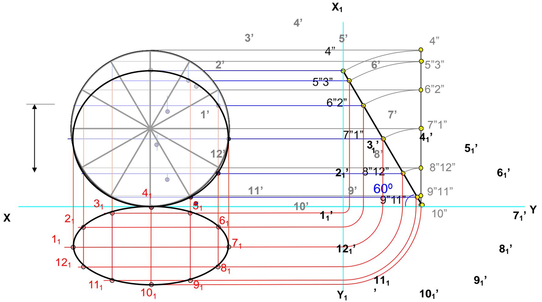
The top view of a plate, the surface of which is inclined at  $60^\circ$  to the HP is a circle of 60 mm diameter. Draw its three views.
