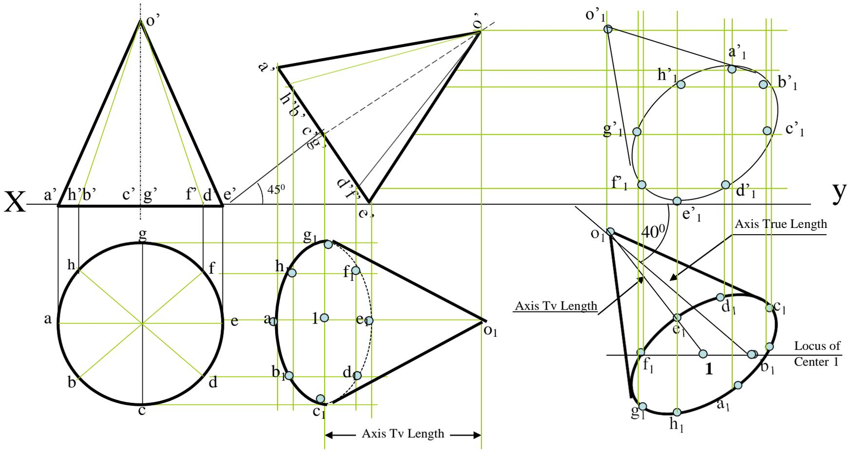
**Problem 10:** A triangular prism, 40 mm base side 60 mm axis is lying on Hp on one rectangular face with axis perpendicular to Vp. One square pyramid is leaning on it's face centrally with axis // to vp. It's base side is 30 mm & axis is 60 mm long resting on Hp on one edge of base. Draw FV & TV of both solids. Project another FV on an AVP 45° inclined to VP.
