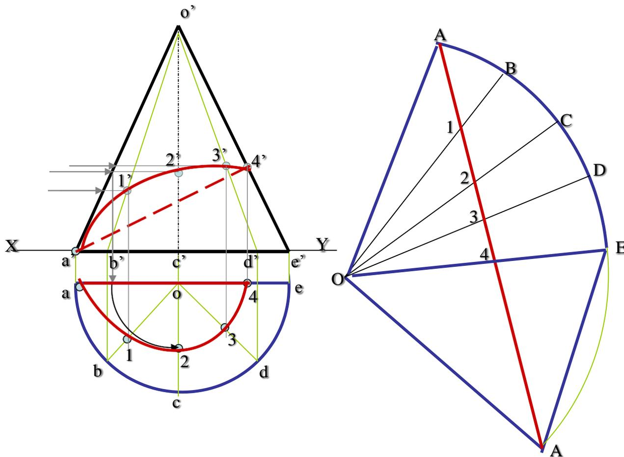
Q 15.26: draw the projections of a cone resting on the ground on its base and show on them, the shortest path by which a point P, starting from a point on the circumference of the base and moving around the cone will return to the same point. Base of cone 65 mm diameter ; axis 75 mm long.
