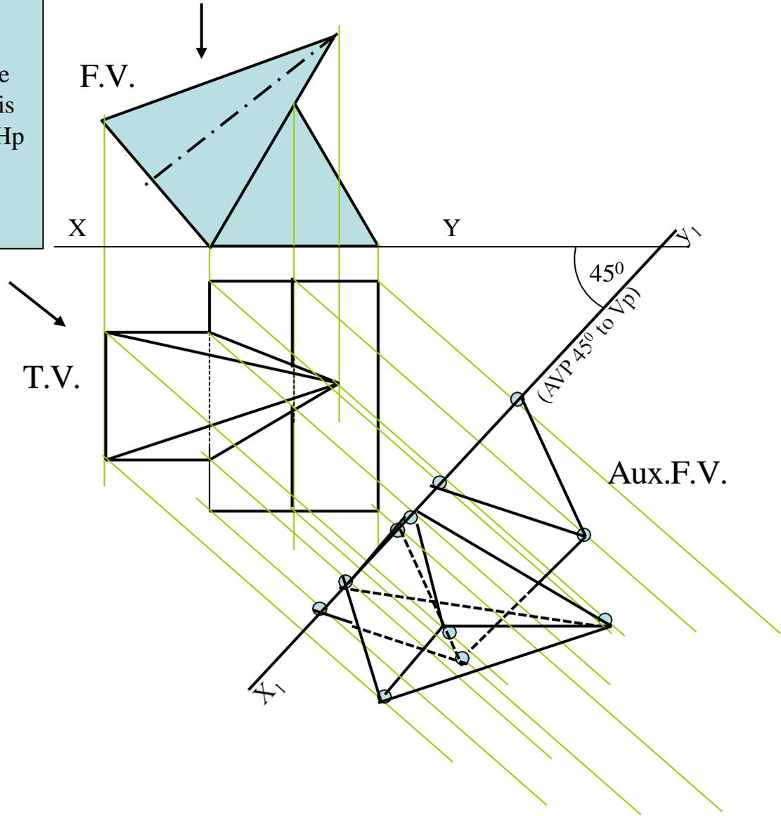
**Problem 11:** A hexagonal prism of base side 30 mm long and axis 40 mm long, is standing on Hp on its base with one base edge // to Vp. A tetrahedron is placed centrally on the top of it. The base of tetrahedron is a triangle formed by joining alternate corners of top of prism. Draw projections of both solids. Project an auxiliary Tv on AIP  $45^\circ$  inclined to Hp.
