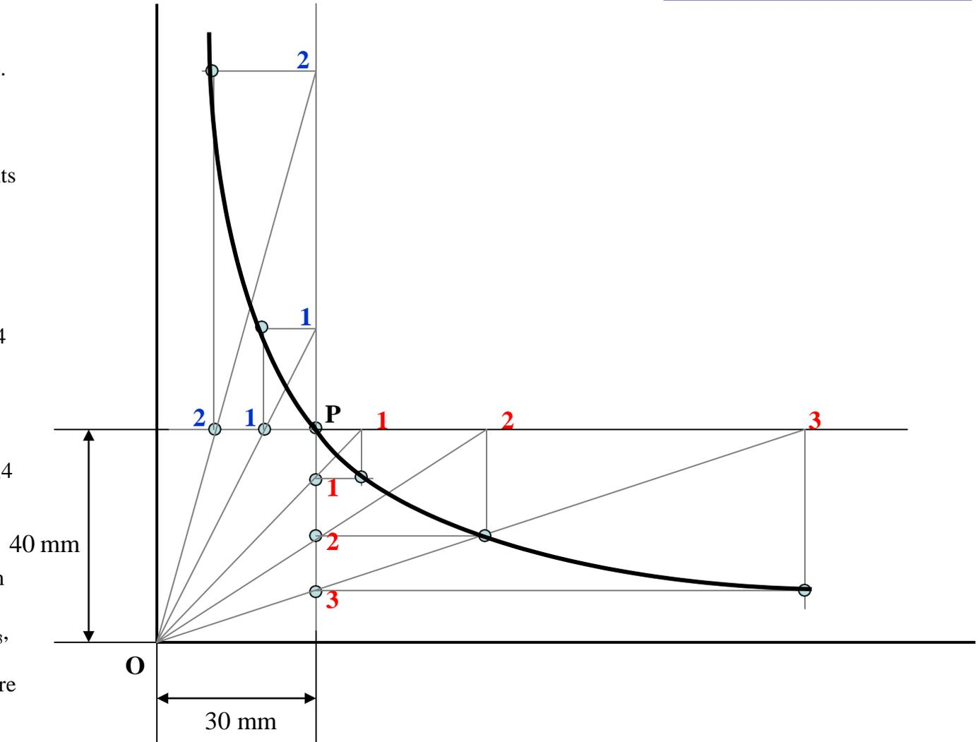
**Problem no.11:** A sample of gas is expanded in a cylinder from 10 unit pressure to 1 unit pressure. Expansion follows law  $PV=Constant$ . If initial volume being 1 unit, draw the curve of expansion. Also Name the curve.
