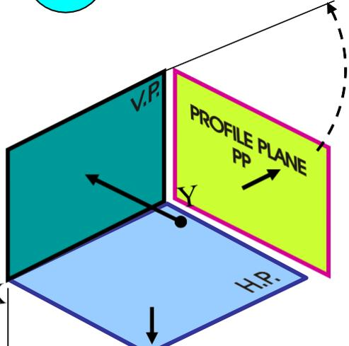
THIS IS A PICTORIAL SET-UP OF ALL THREE PLANES. ARROW DIRECTION IS A NORMAL WAY OF OBSERVING THE OBJECT. BUT IN THIS DIRECTION ONLY VP AND A VIEW ON IT (FV) CAN BE SEEN. THE OTHER PLANES AND VIEWS ON THOSE CAN NOT BE SEEN.
