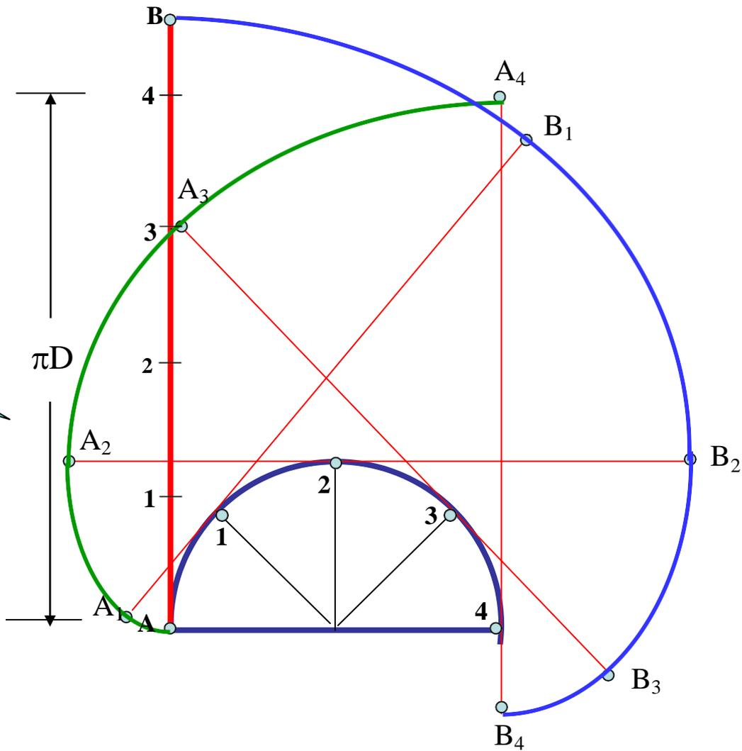
**Problem 22:** Draw locus of a point on the periphery of a circle which rolls on straight line path. Take circle diameter as 50 mm. Draw normal and tangent on the curve at a point 40 mm above the directing line.
