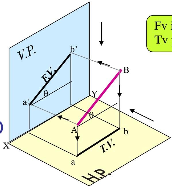
Fv inclined to xy
