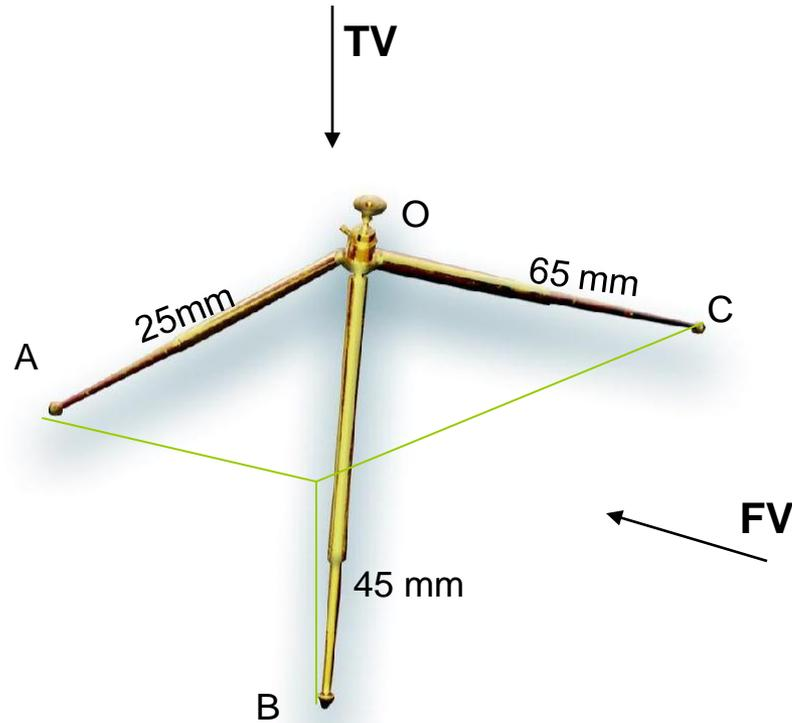
**PROBLEM 17:-** A pipe line from point **A** has a downward gradient 1:5 and it runs due East-South. Another Point **B** is 12 M from **A** and due East of **A** and in same level of **A**. Pipe line from **B** runs  $20^\circ$  Due East of South and meets pipe line from **A** at point **C**. Draw projections and find length of pipe line from **B** and its inclination with ground.
