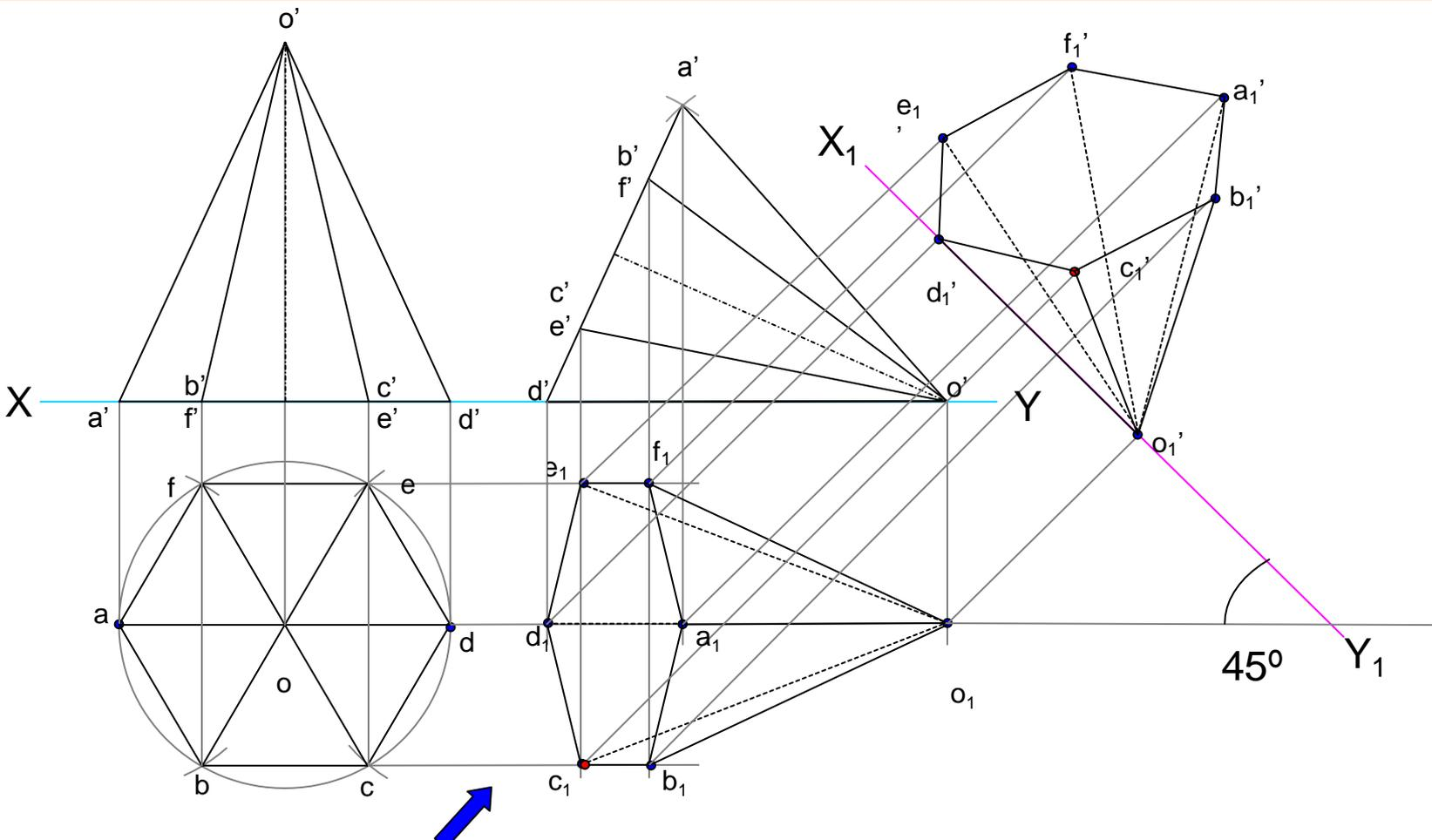
**Problem 5:** A cube of 50 mm long edges is so placed on HP on one corner that a body diagonal is parallel to HP and perpendicular to VP. Draw its projections.
