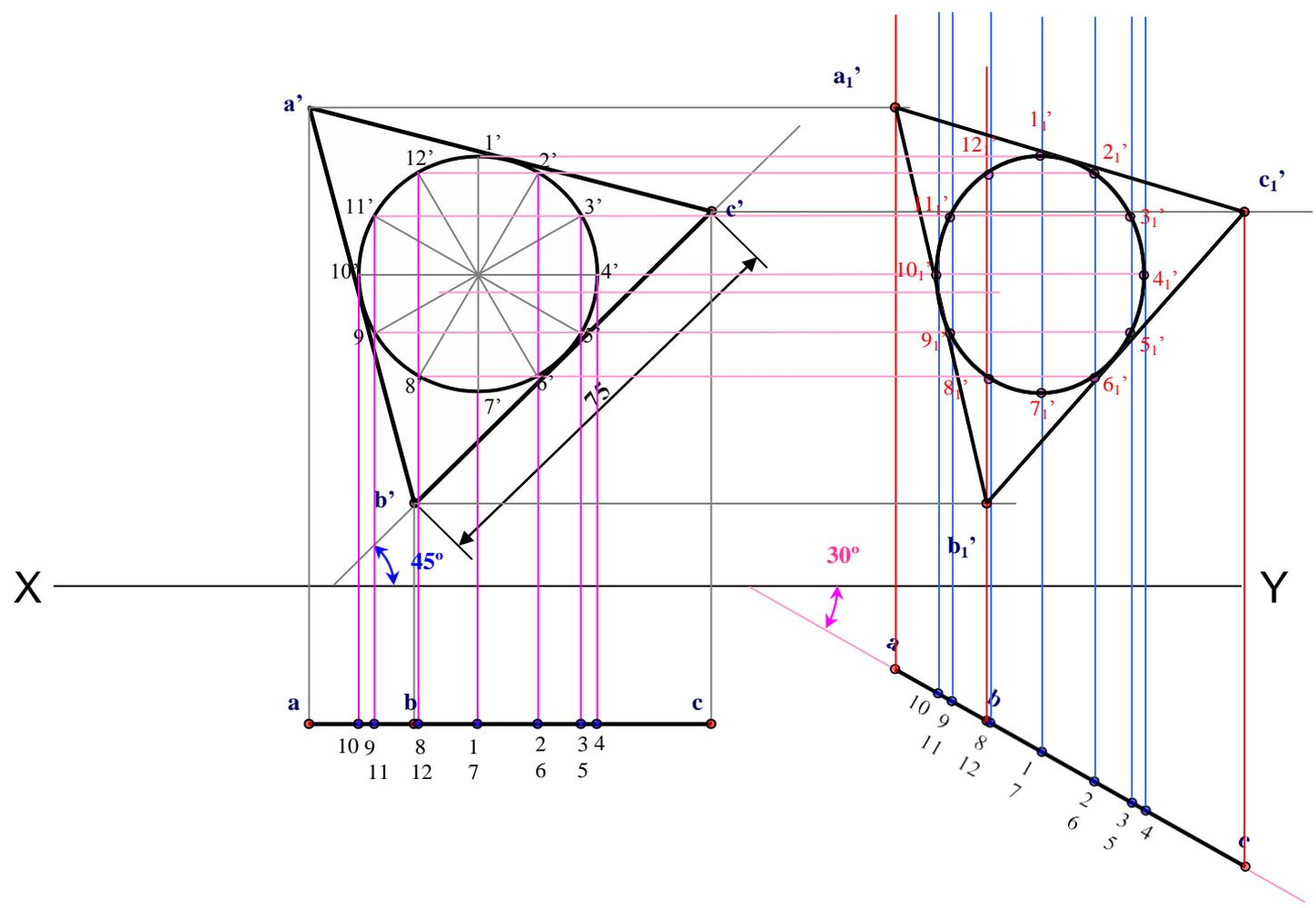
**Q12.7: Draw the projections of a regular hexagon of 25mm sides, having one of its side in the H.P. and inclined at  $60^\circ$  to the V.P. and its surface making an angle of  $45^\circ$  with the H.P.**
