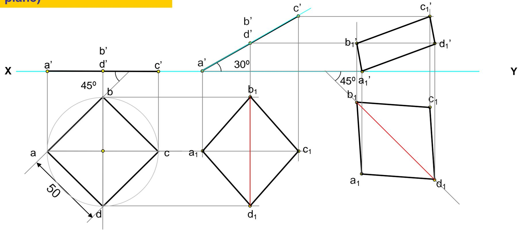
**Q: Draw a rhombus of 100 mm and 60 mm long diagonals with longer diagonal horizontal. The figure is the top view of a square having 100 mm long diagonals. Draw its front view.**
