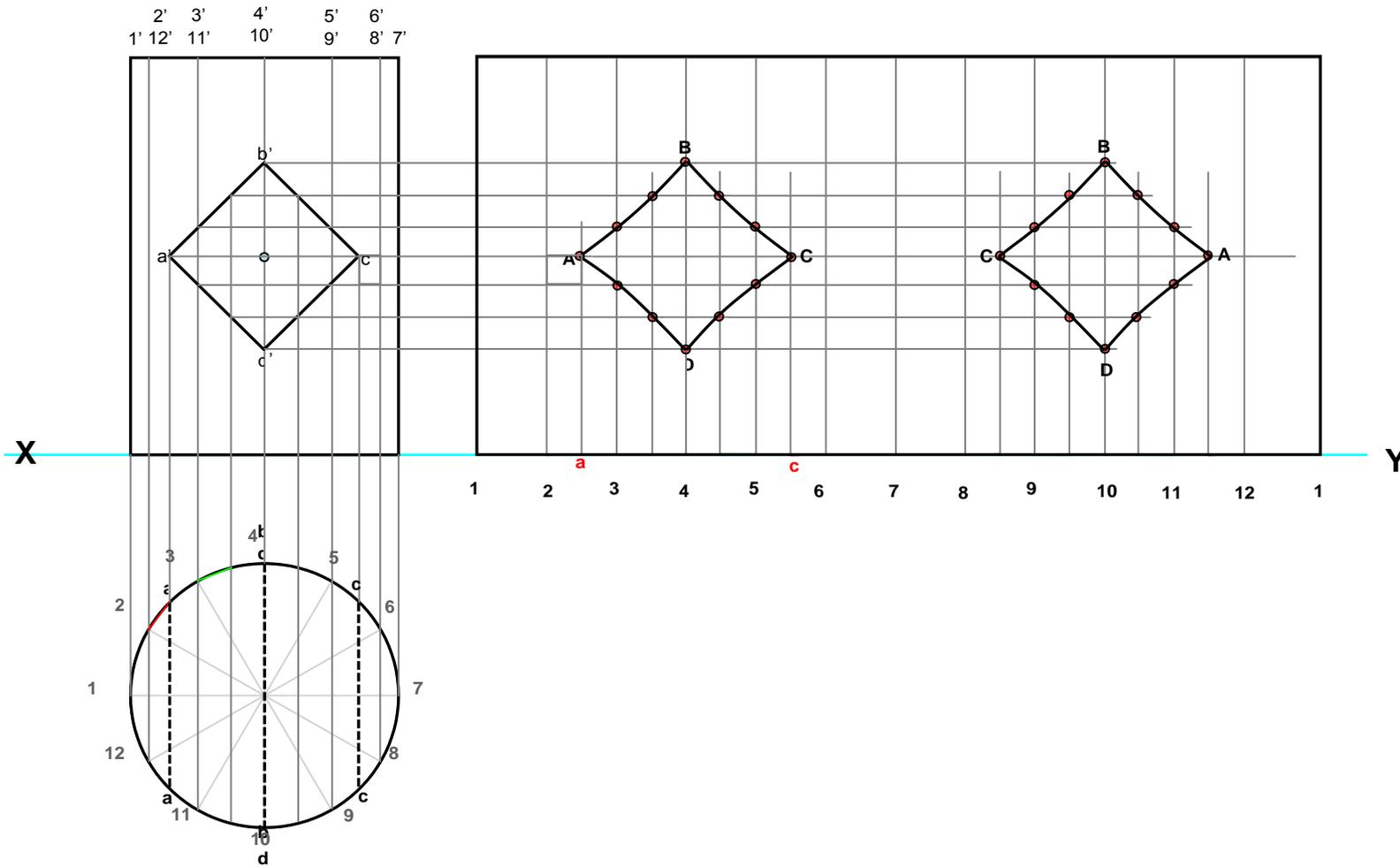
**Q.15.21: A frustum of square pyramid has its base 50 mm side, top 25 mm side and axis 75 mm. Draw the development of its lateral surface. Also draw the projections of the frustum (when its axis is vertical and a side of its base is parallel to the VP), showing the line joining the mid point of a top edge of one face with the mid point of the bottom edge of the opposite face, by the shortest distance.**
