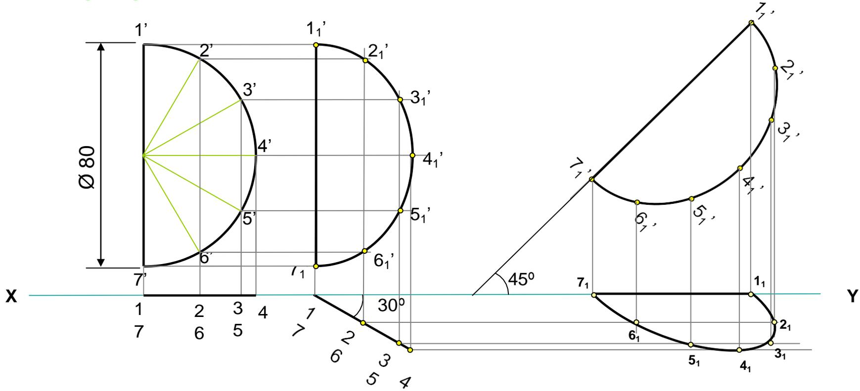
**Problem 12.8 :** Draw the projections of a circle of 50 mm diameter resting on the HP on point A on the circumference. Its plane inclined at  $45^\circ$  to the HP and (a) The top view of the diameter AB making  $30^\circ$  angle with the VP (b) The the diameter AB making  $30^\circ$  angle with the VP
