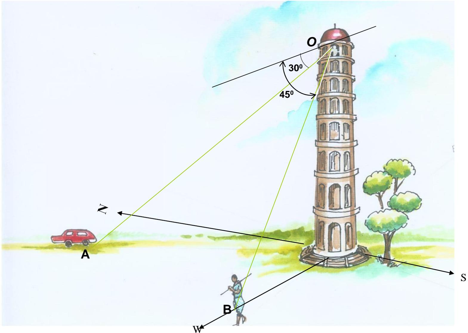
**PROBLEM 19:-** Guy ropes of two poles fixed at 4.5m and 7.5 m above ground, are attached to a corner of a building 15 M high, make 30° and 45° inclinations with ground respectively. The poles are 10 M apart. Determine by drawing their projections, Length of each rope and distance of poles from building.
