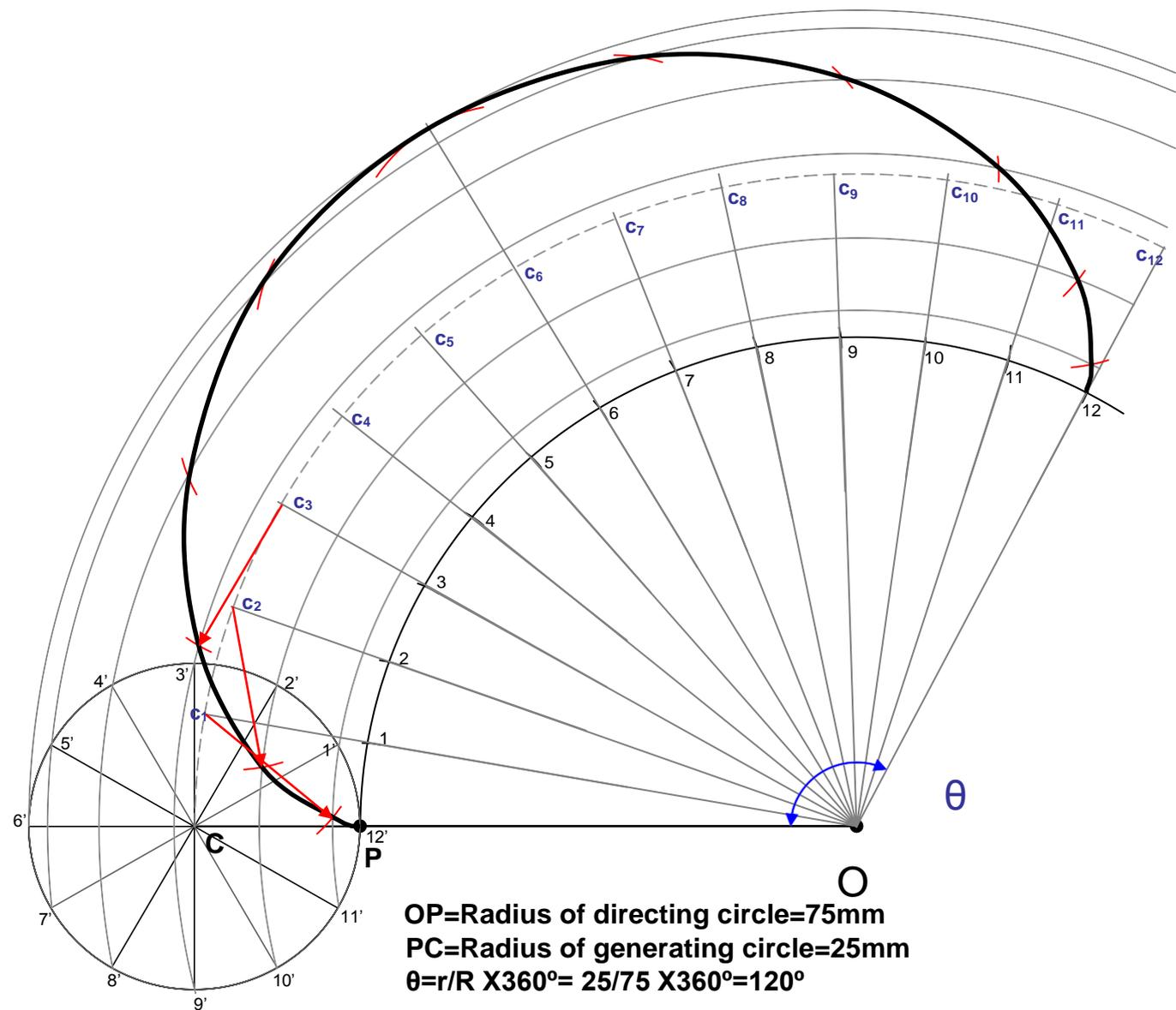
**PROBLEM 26:** DRAW LOCUS OF A POINT ON THE PERIPHERY OF A CIRCLE WHICH ROLLS FROM THE INSIDE OF A CURVED PATH. Take diameter of rolling circle 50 mm and radius of directing circle (curved path) 75 mm.
