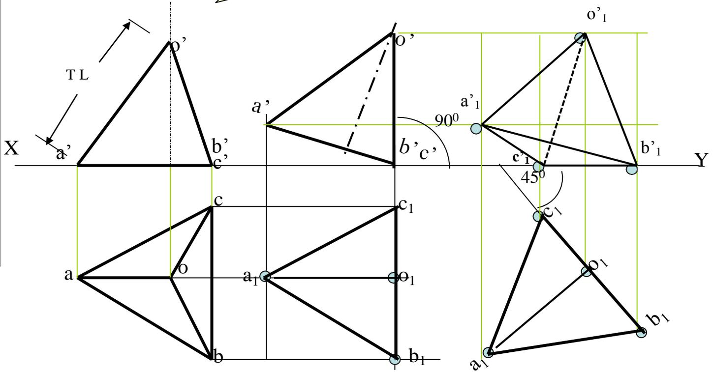
**Problem 1.** A square pyramid, 40 mm base sides and axis 60 mm long, has a triangular face on the ground and the vertical plane containing the axis makes an angle of  $45^\circ$  with the VP. Draw its projections. Take apex nearer to VP
