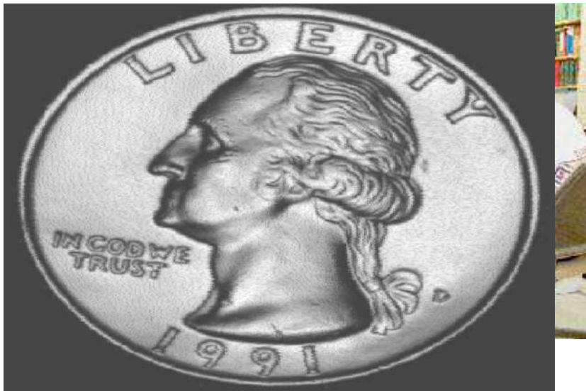
Gray scale image produced using the sound reflected from the front surface of the coin
