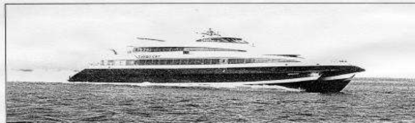
FIGURE 2: 45 m Tri Cat fast catamaran ferry built by FBM Marine Ltd.
