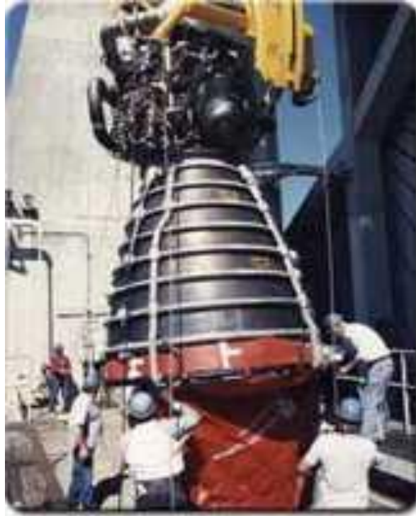
Main Engine Space Shuttle 374,000 lbs thrust (SL) LOX/H 2
