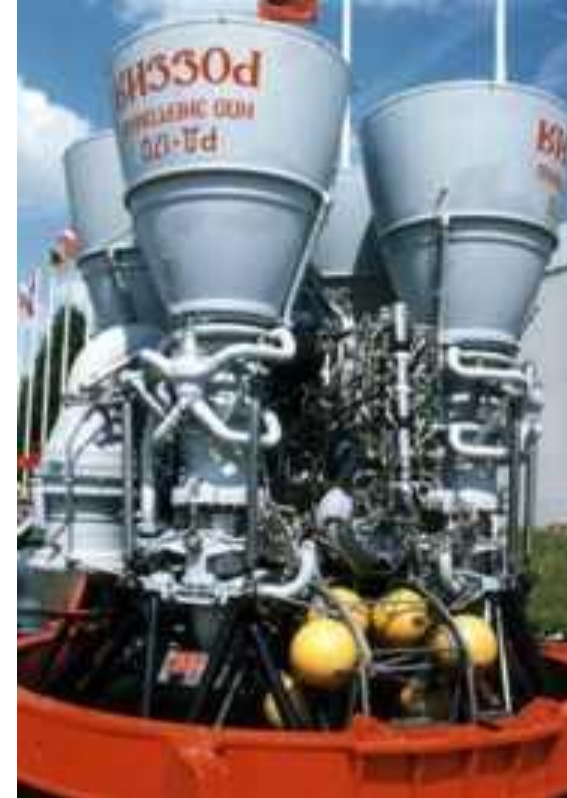
RD-170 1.78 million lbs thrust (SL) LOX/Kerosene
