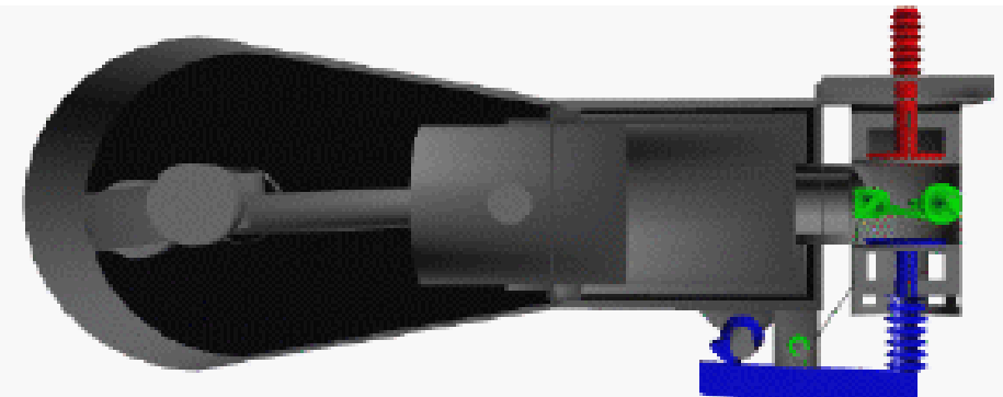
Stage 6 – Begin Exhaust Stroke
