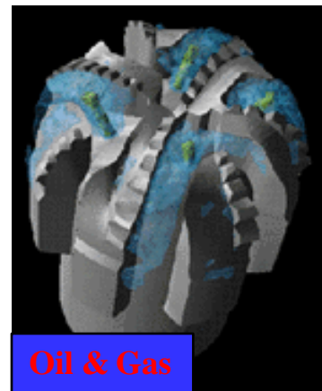
Flow of lubricating mud over drill bit
