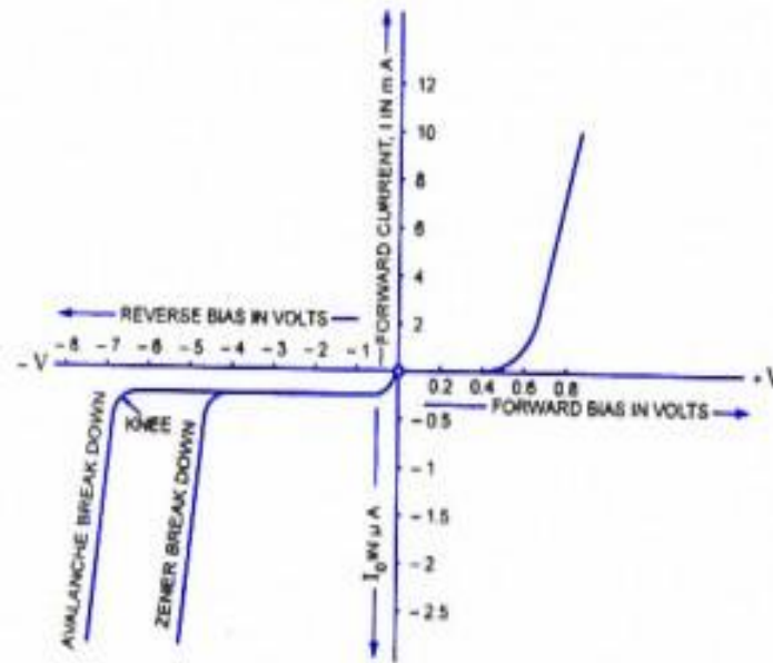
Fig.19: avalanche breakdown and Zener breakdown.
