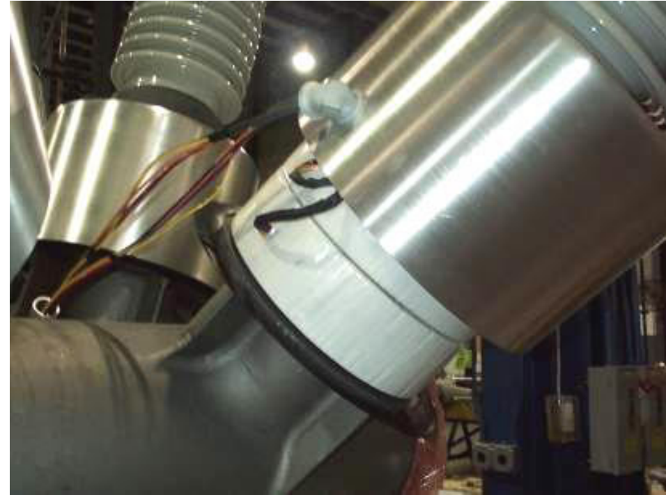
Polyester Taped Bushing CT on Outdoor Circuit Breaker
