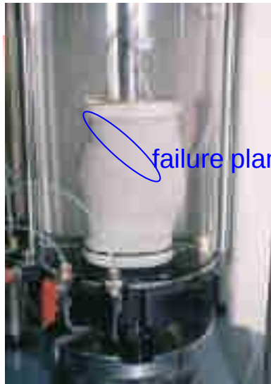
soil sample at failure
